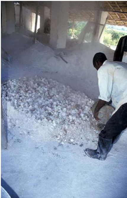
Figure 3: Hydrating of quicklime using a watering can Chenkumbi Limeworks, Malawi © Practical Action/Dave Mather
