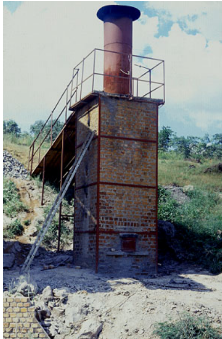
Figure 2: A vertical shaft kiln for small-scale production of lime. Chegutu, Zimbabwe. ©Practical Action/Kelvin Mason
