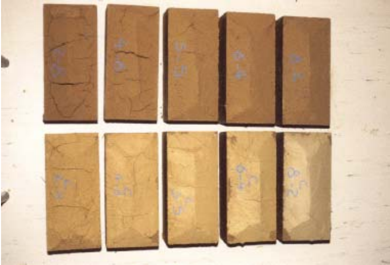
Figure 3: Test carried out on unstabilised and stabilised mortars to determine the soil/sand ratio ©CRATerre/EAG
