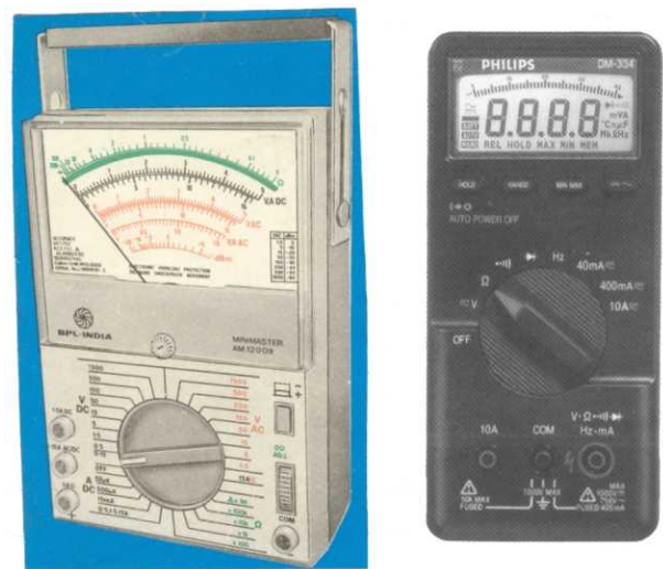
Fig. 1.5 (a) Analog Multimeter (BPL). (b) Digital Multimeter (Philips).
