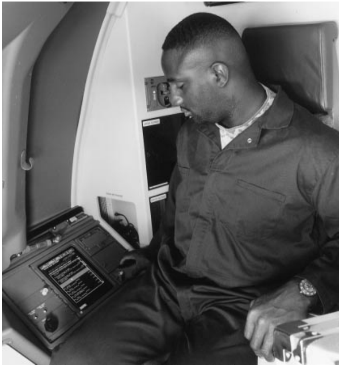
Figure 12. Boeing 777 maintenance access terminal.
