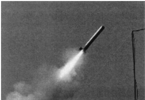
Figure 20. NATO Sea Gnat MK-216 distraction decoy deployed from a rocket launcher.
