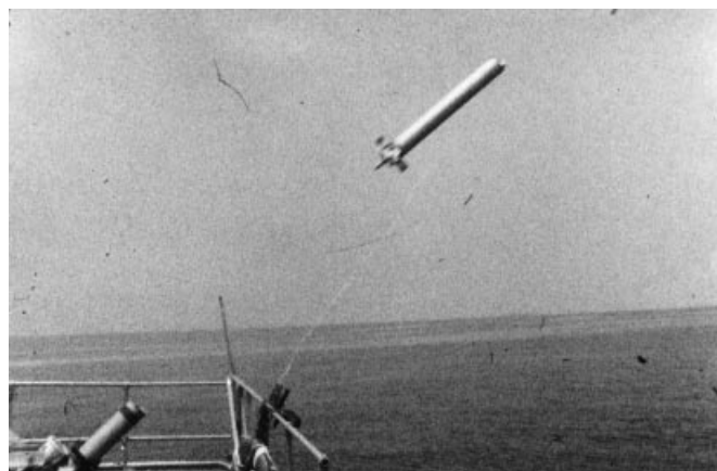
Figure 17. NATO Sea Gnat MK-214 seduction RF decoy deployed from a shipboard rocket launcher.
