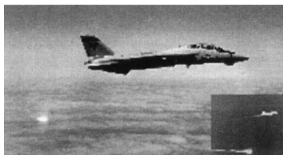
Figure 27. Flare IR decoy deployed from a tactical aircraft in flight.
