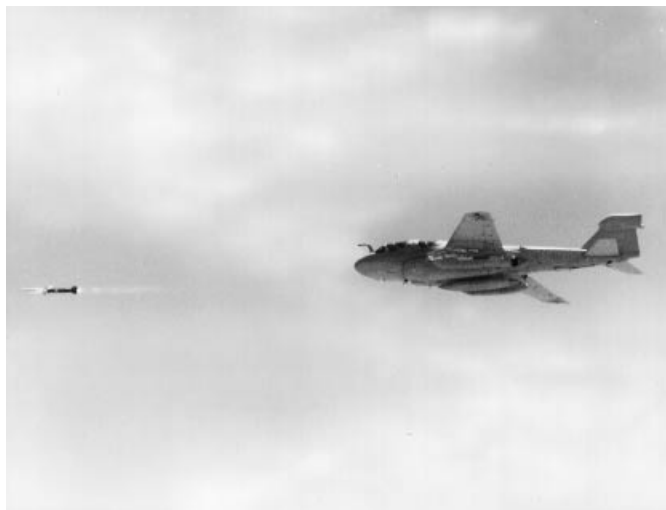
Figure 4. HARM missile (shown after separation from an EA-6B aircraft) is an EW weapon for physically destroying the source of hostile radiation.
