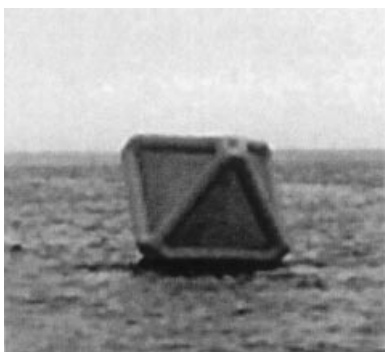
Figure 19. AN/SLQ-49 inflatable corner reflector decoy deployed at sea.
