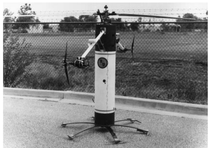
Figure 23. EAGER shipboard-tethered decoy in field trials.
