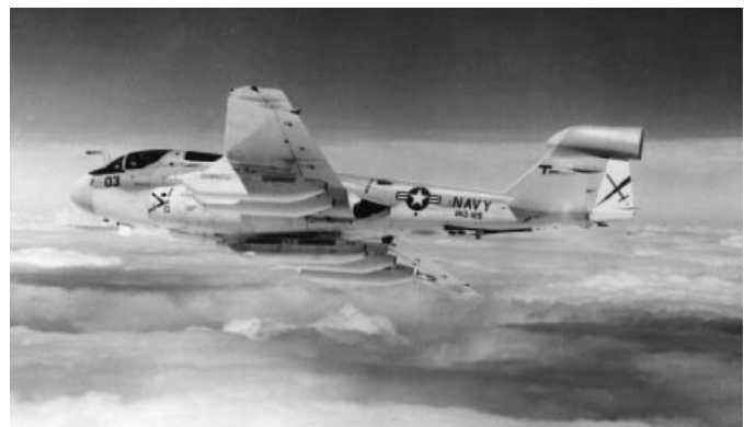
Figure 11. EA-6B aircraft equipped with the AN/ALQ-99 EA system for airborne CTAR.
