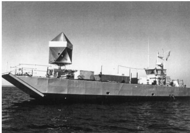
Figure 26. Multifaceted corner reflector deployed on a ship bow to provide a high cross-sectional reflection at several frequencies.
