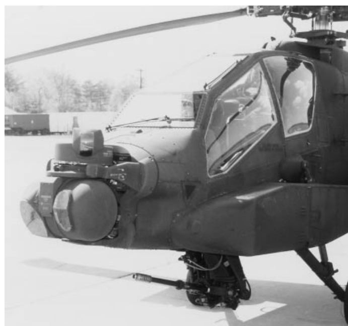
Figure 4. The PNVS thermal imager mounted on the front of the Apache Helicopter. The TADS system is the barrel-shaped object with two windows mounted beneath the PNVS.
