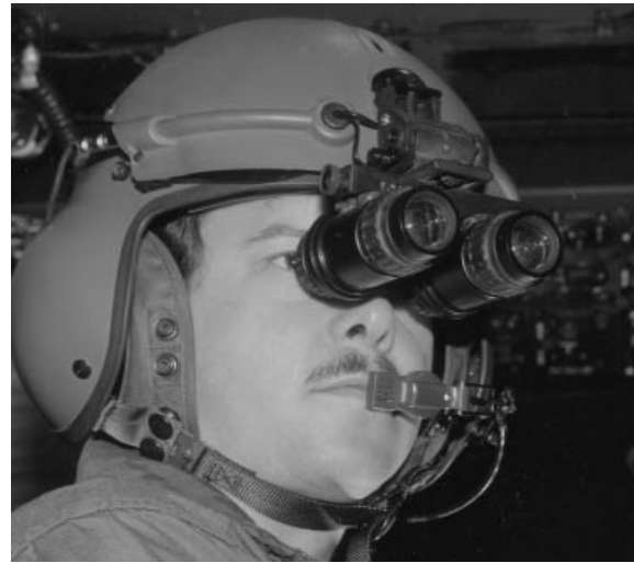
Figure 2. The ANVIS goggle provides a good image with moonlight or starlight illumination. The pilot can view instruments by looking under the goggle.
