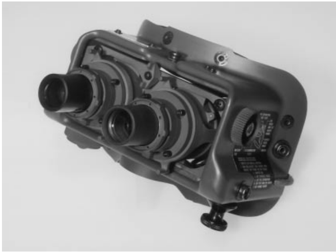
Figure 1. The AN/PVS-5 goggle provides a good image with moonlight illumination. In use, it covers the entire upper portion of the face.
