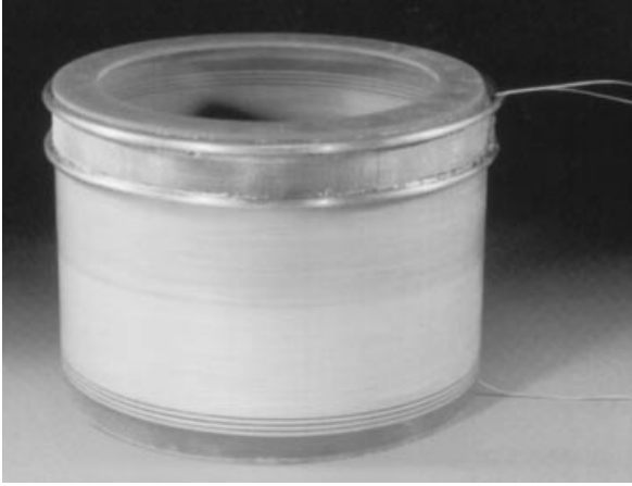
Figure 5. Model coil made by ABB, from wire provided by American Superconductor Corporation, for the 630 kVA transformer project in Geneva, Switzerland.
