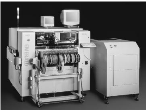
Figure 5. Example of flexible placement machine. (Figure of Philips Eclipse courtesy of North American Philips.)
