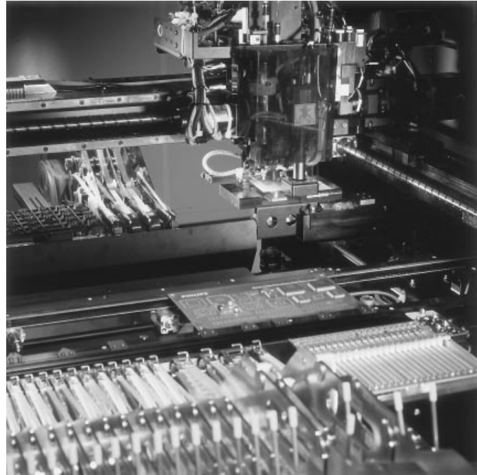
Figure 2. Example of placement mechanism of fine pitch equipment with flexible placement head. (Figure of Philips Eclipse courtesy of North American Philips.)
