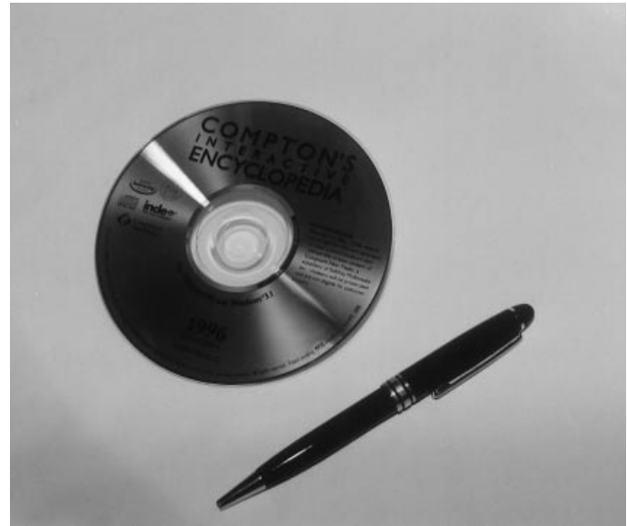
Figure 1. A CD-ROM disk is 120 mm in diameter and can hold up to 650 Mbytes of information.
