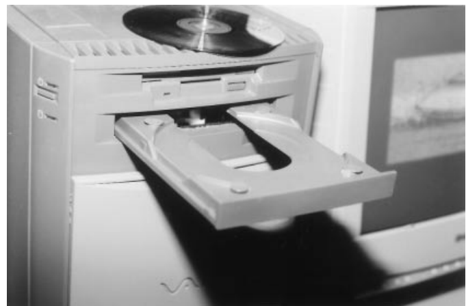
Figure 2. A CD-ROM drive (player) is a common component of most new personal computers.
