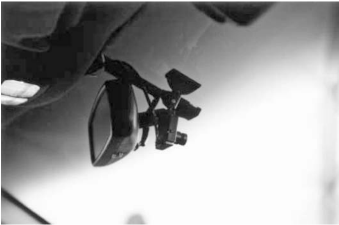
Figure 7. The steering control system uses a small camera mounted on the windshield. Photo by Robert Bryant, Avalon Integrated Services.
