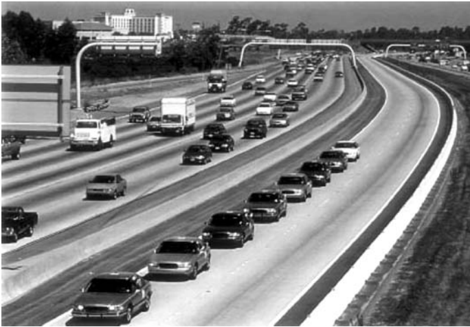
Figure 1. A platoon of eight automated cars moving on the I-15 high-occupancy vehicle (HOV) lanes during the AHS demonstration in San Diego. Photo by Bill Stone, California PATH.
