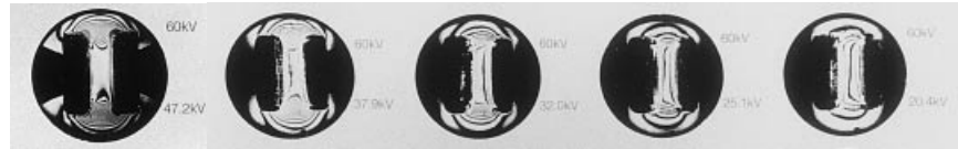
Figure 17. Kerr electrooptic fringe patterns in ethylene carbonate at T = 42.9^\circ\text{C} with resistivity \sim 4 \text{ M}\Omega\text{-cm} at early ( \sim 20 \mu\text{s} ) and long times (1, 2, 3 and 4 ms) after charging from a Marx generator at 60 kV with stainless steel electrodes of length 35 cm and gap of 1 cm. At early time ( \sim 20 \mu\text{s} ), the uniform light intensity in the central interelectrode region indicates the space-charge free uniform electric field, while the interelectrode fringes at longer times indicate significant positive charge injection. The 60 kV charging voltage is given in the upper right, while the instantaneous voltage is given at the lower right of each photograph. E_m \approx 8.3 \text{ kV/cm} .
