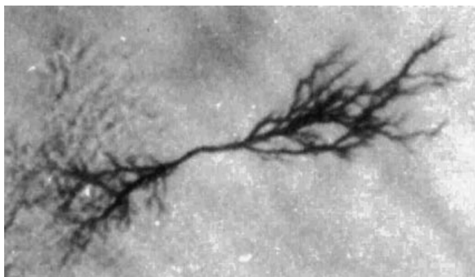
Figure 3. Bow-tie electrical tree with filaments, in the direction of the electric field, at a defect in polymeric insulation.
