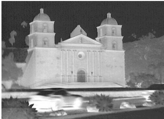
Figure 5. Single frame of night imagery of Mission Santa Barbara obtained with Hughes LWSS portable uncooled sensor. (From Hughes Santa Barbara Research Center, with permission, © 1997, Santa Barbara Research Center.)
