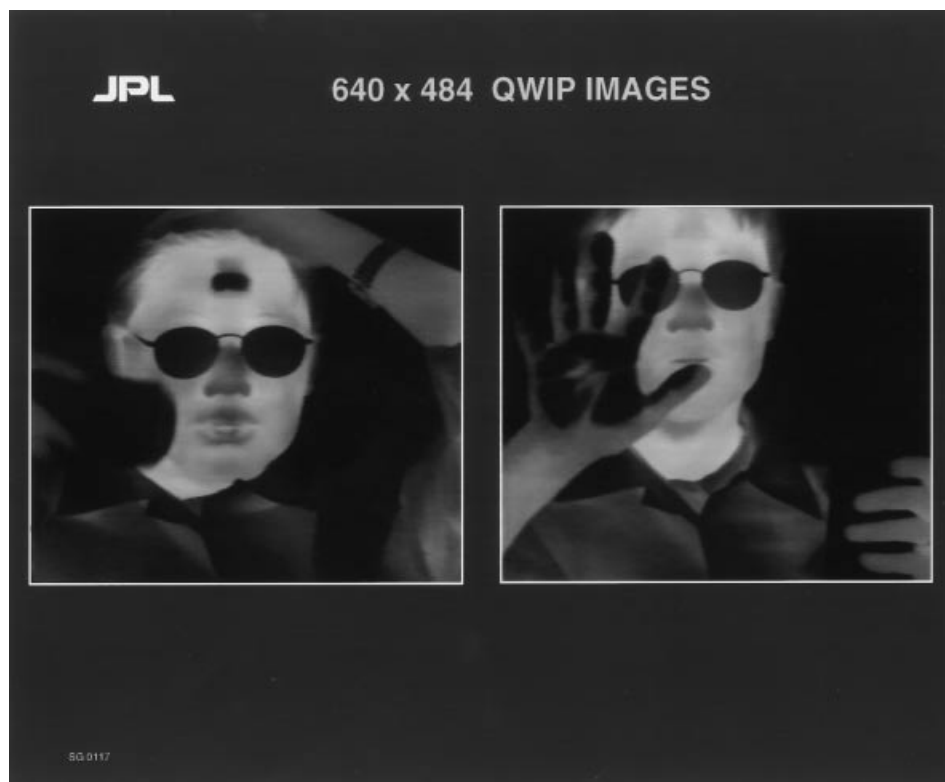
Figure 14. Images taken with a QWIP camera having 640 \times 484 pixels. Illustration courtesy of JPL (14).
