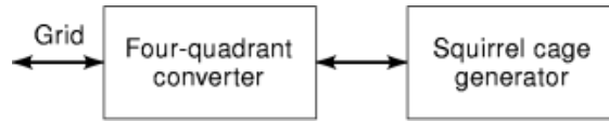
Fig. 9. Squirrel cage induction machine with a four-quadrant power converter used for producing constant output frequency from a variable-speed prime mover.
