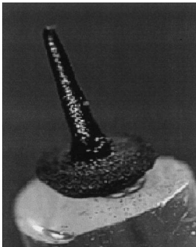
Figure 17. Micrograph of a 700 \mu\text{m} tall solid rod of SiC grown from gas phase using a focused diode laser beam inside a sealed chamber containing tetramethylsilane.
