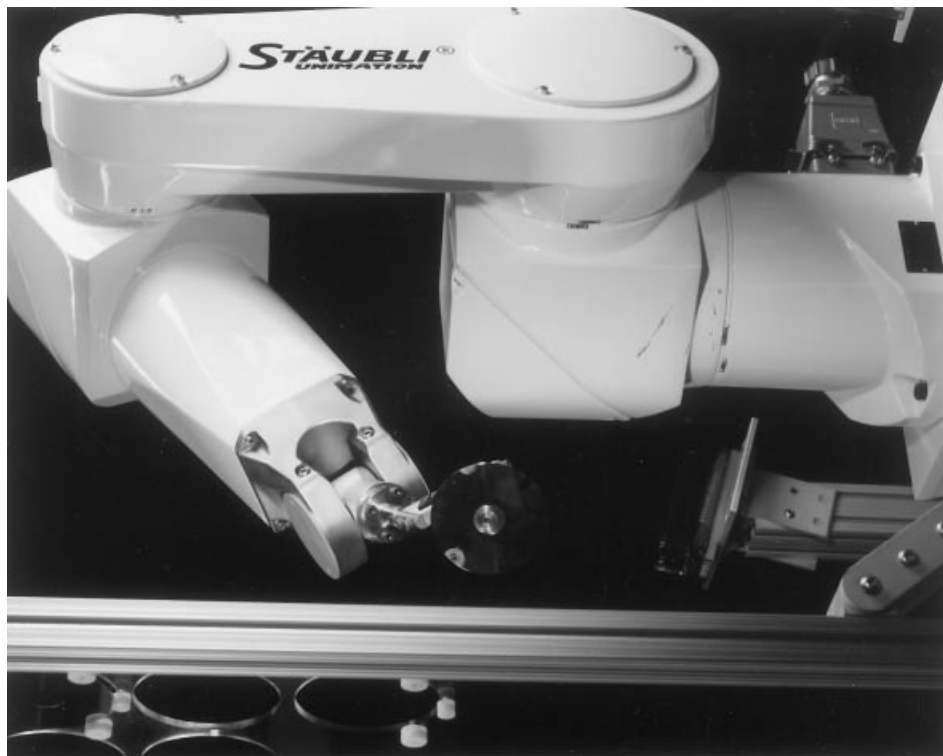
Figure 8. Clean room applications include wafer handling and sputtering. Courtesy of Staubli Unimation, Duncan S.C.
