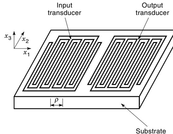
**Figure 1.** SAW delay line consisting of two interdigital transducers on a piezoelectric substrate.
