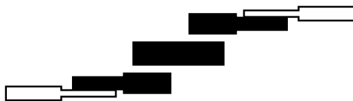
Figure 57. Multilayer parallel coupled-line filter. Various conductors can be placed on different levels; each coupled section produces tight coupling, leading to broad bandwidth for the filter.
