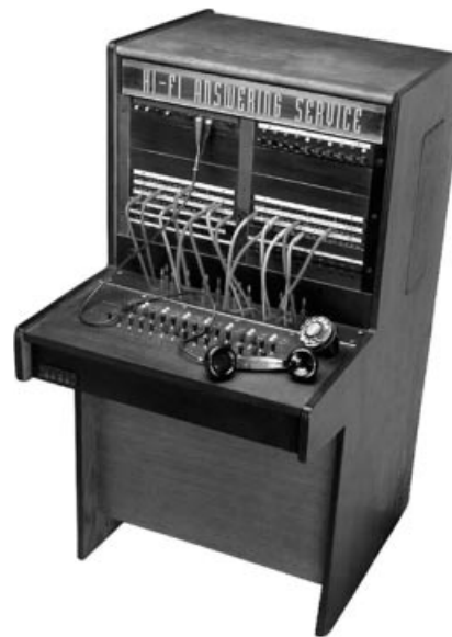
Figure 1. Example of an early manual switchboard. (Copyright 1997. Reprinted by permission of Classic P10 Partners.)
