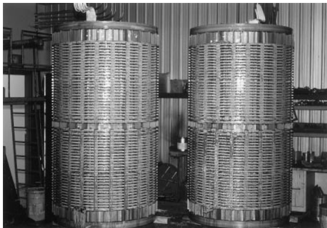
Figure 8. Photograph of two coils of a 10 MVA, 25 kV/6.9 kV transformer after impregnation. Courtesy of Megatran Electric Ltd., St-Jean-sur-Richelieu, QC, Canada.
