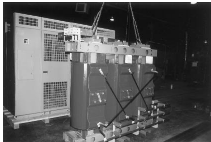
Figure 10. Photograph of the core and enclosure of a 5 MVA, 25 kV/600 V cast-coil transformer. Courtesy of Megatran Electric Ltd., St-Jean-sur-Richelieu, QC, Canada.
