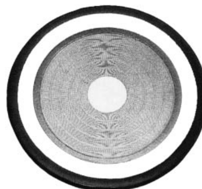
Figure 18. A top view of the reverse conducting GTO thyristor (4500 V, 3000 A) (23). The diode is located at the periphery of the device.
