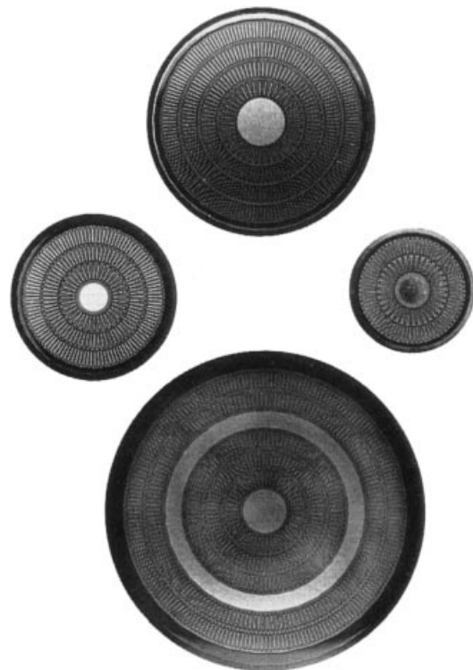
Figure 11. Typical GTO thyristor basic segment arrays (19), with a multi-emitter structure corresponding to the current carrying capability. An important design point for large current GTO thyristors is how to prevent current crowding during turn-off operation.
