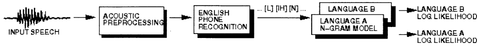
Figure 4. The phone recognition followed by phone frequency and phone sequence language modeling LID system. Phone recognition is performed in one language, in this case, English. Phone frequency and sequence statistics are used to determine the language of the speech utterance.
