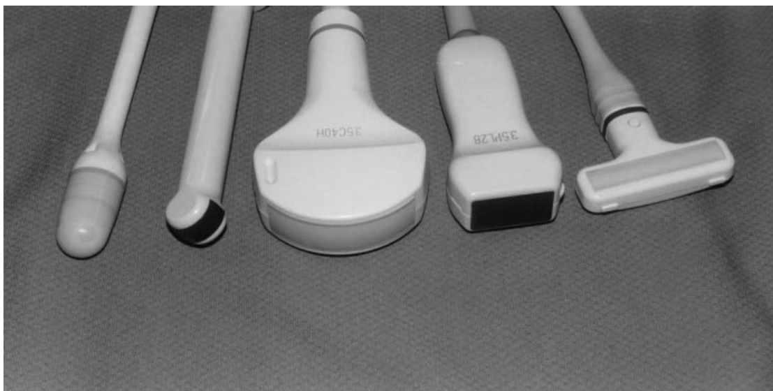
Figure 1. Representative types of medical imaging transducers. From left: a mechanically scanned and a strongly curved linear array endoscopes, a curved linear array, a linear phased array, and a side-looking linear array for imaging during surgery. (Courtesy of Siemens Medical Systems, Inc. Ultrasound Group)
