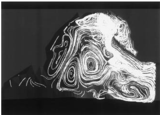
Figure 10. Streamlines in a stationary velocity field. (Data from Delft Hydraulics.)
