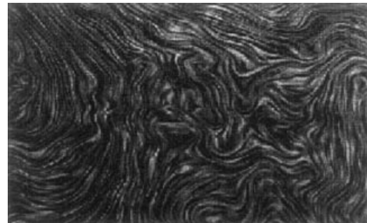
Figure 15. Spot noise applied to a 2-D slice of a 3-D simulation of the flow around a square block. The section behind the block is shown. (Simulation is by R. W. C. P. Verstappen and A. E. P. Veltman, University of Groningen, The Netherlands; Visualization is by W. de Leeuw, Center for Mathematics and Computer Science (CWI), Amsterdam.)
