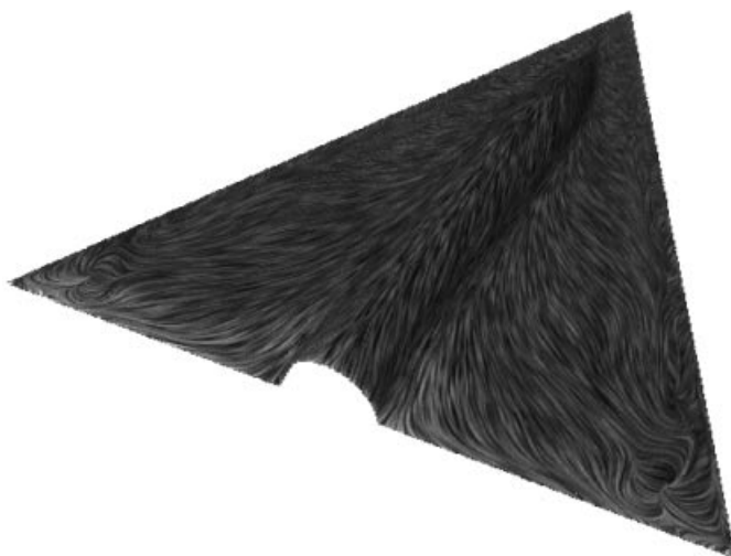
Figure 14. LIC applied to a delta wing simulation. (Data courtesy of Neal Chaderjian, visualization is by David Kao, NASA Ames Research Center.)
