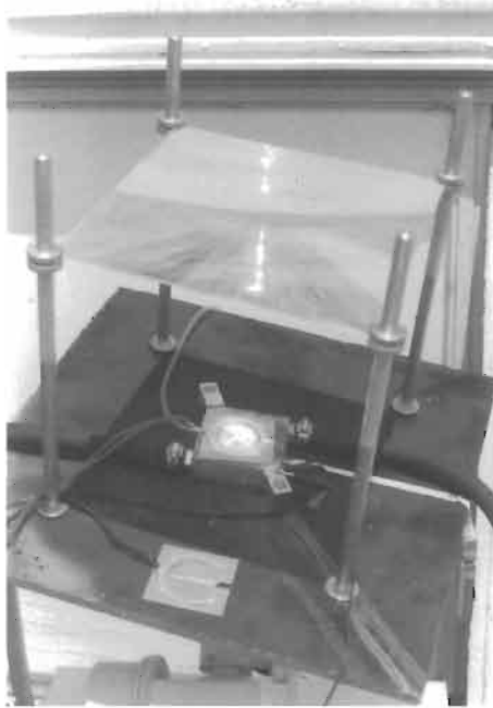
Figure 7 Concentrator test setup showing the principal sub-systems: lens, cell and heat sink (here actively cooled with water). Note that the cell requires suitable thermal and electrical connectors. (IES, 1978).
