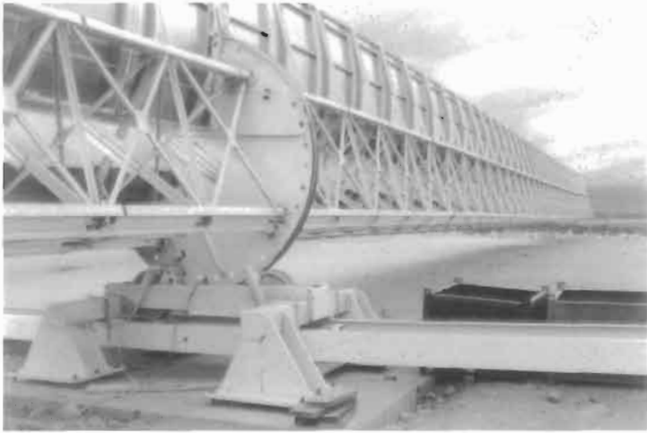
Figure 15 A close-up view of a large tracking driver for a single-axis tracking system. The mechanism can carry up to 2000 N and provide a position accuracy of \pm 0.05^\circ . The accuracy of the driver is derated by the mechanical deformation of the structure, allowing only \pm 0.2^\circ (EUCLIDES-THERMIE Plant, Tenerife, 1998).
