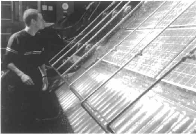
Figure 7 Shell PV roof undergoing 'Prescript' test in Solar Simulator at Cardiff, UK.
