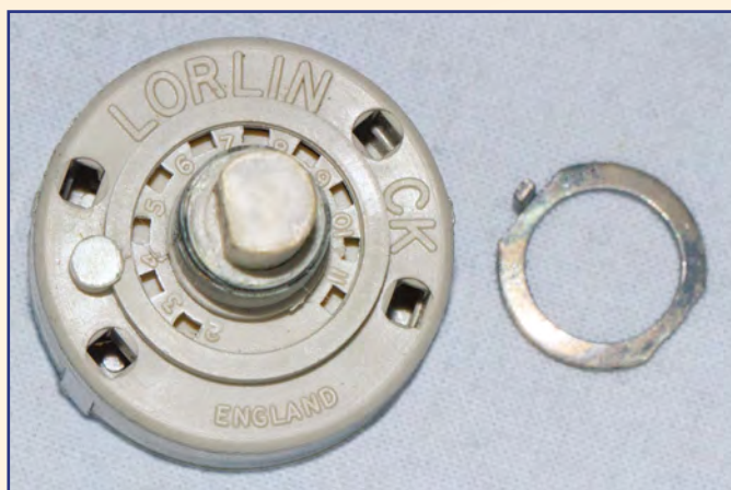
Fig.3. Many rotary switches have an adjustable end-stop that can handle anything from 2 to 11-way operation. It is omitted if 12-way operation is required
