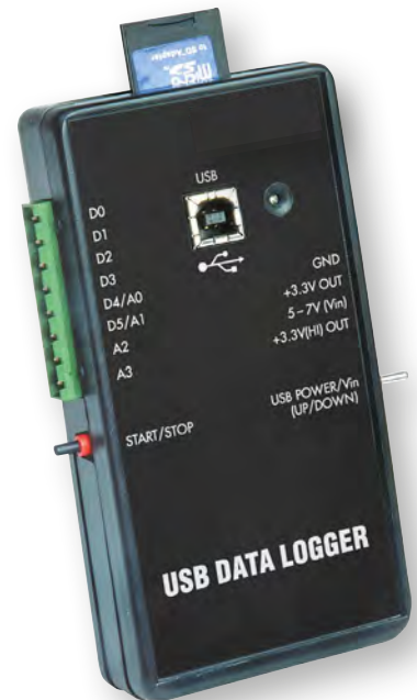
This view shows the completed USB Data Logger with the memory card plugged in
