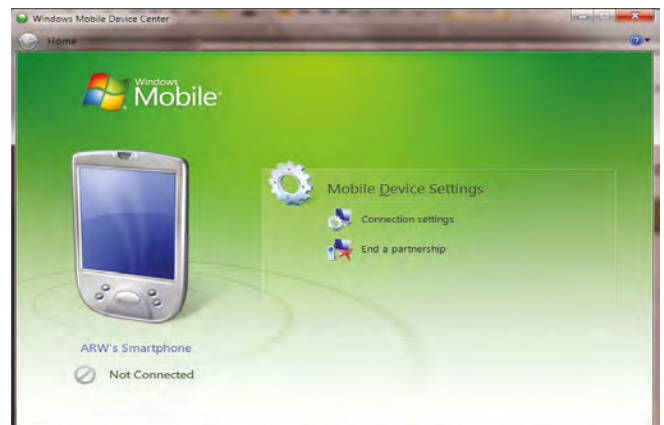
W7 Mobile Device Centre settings: showing as 'Not Connected', which will allow Internet sharing
