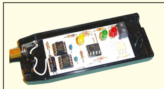
PCB assembled in the lower case half. Note the probe solder tag and white lead to the circuit board
