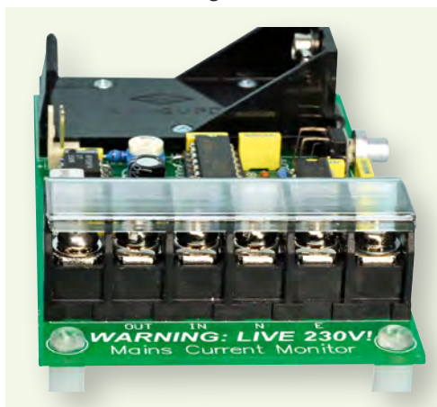
Two M3 × 10mm tapped nylon spacers are fitted to one end of the PCB as supports.
