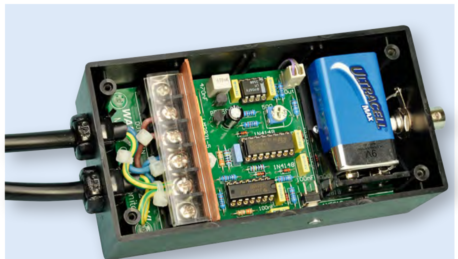
The unit all wired up and ready to go. Note how the 2-wire ribbon cable for the output signal is clamped by the PCB. There isn't a lot of room for the output connector next to the battery, so we had to trim its central solder pin. You can also see how the Presspahn cover is held in place by the plastic case slots, terminal block and tapped spacer.
