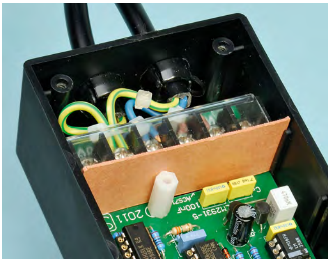
This close-up view shows how the Presspahn cover is held in place by the plastic case slots, the mains terminal block and the M3 × 15mm tapped spacer.
