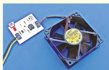
Fig.24. Most large PC fans will operate with a supply of between 9V and 12V and currents of 150-300mA
