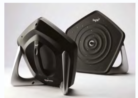
Front and rear of the KAIST sound camera
