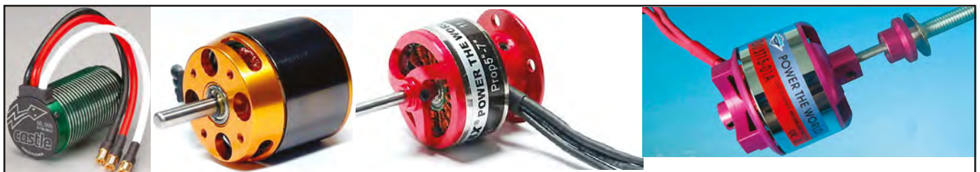
A small selection of the thousands of commercial brushless motors available. They're easily distinguishable from standard (ie brushed) motors because invariably they will have three wires – brushed motors have just two.
