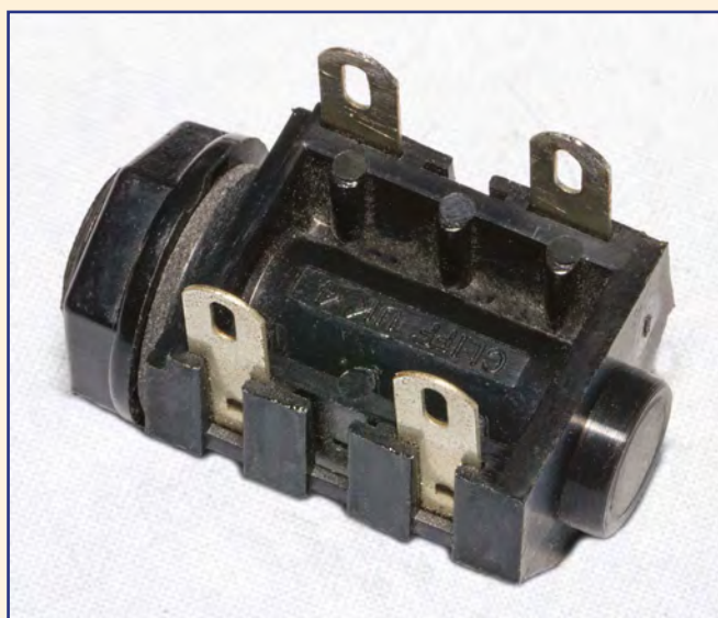
Fig.3. Standard jacks are one of the oldest types of connector, but are still in widespread use today. This is a standard socket that has two built-in switches
