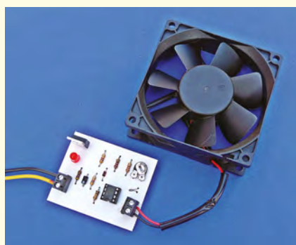
Fig.23. Our Temperature Alarm is ideal for use in cooling applications
