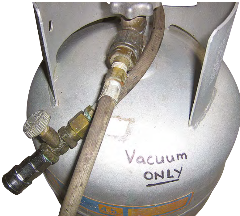
Fig.4: a reservoir tank made from a 9kg gas bottle, adapted to a standard air line fitting. It is worth knowing that most pipe fittings have a BSP (British Standard Pipe) thread. This includes air lines, refrigeration, plumbing, irrigation, it is a fairly universal thread. BSP fittings will even screw into most American (NPT) fittings. Note though that gas lines use a tapering thread (BSPT) while most other pipes use a parallel thread (BSPP).
