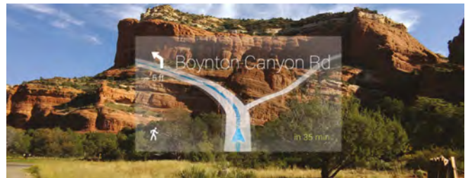
An early example of Google Glass satellite navigation. A mobile phone Bluetooth connection provides GPS and SMS
