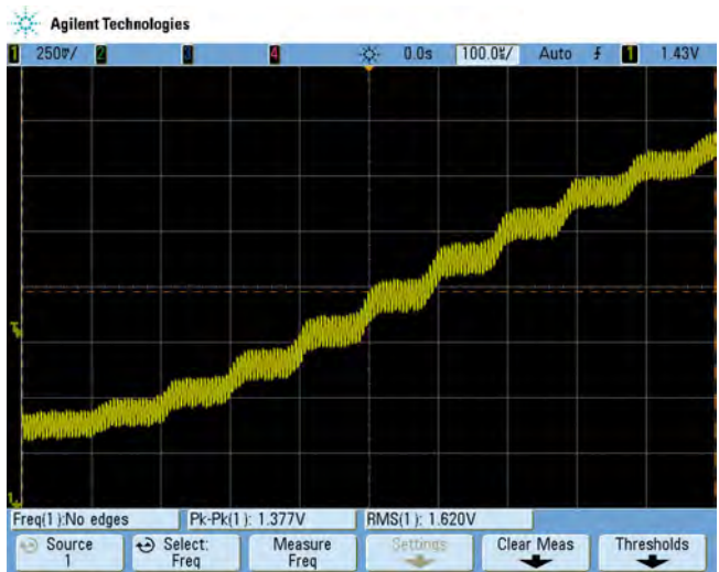
Fig.2(c): the same sinewave (11.025kHz sampling rate) being played back without the linear interpolation code active. The resulting steps cause audible artefacts, especially with lower sampling rates.
