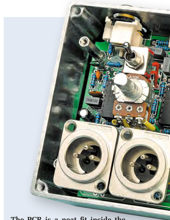
The PCB is a neat fit inside the case. In practice though, it is first attached to the lid before the entire assembly is dropped into place.
