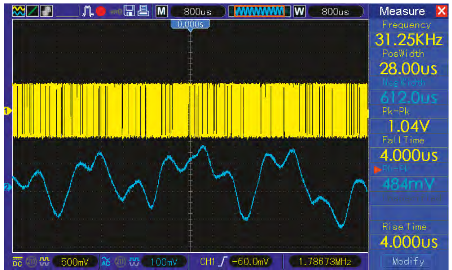
Fig.11: this scope grab compares the S/PDIF digital audio output from the interface (yellow trace) with the analogue audio output waveform (blue trace), when a WAV file is being played back. The timebase here has been slowed down to show the audio waveform clearly.
