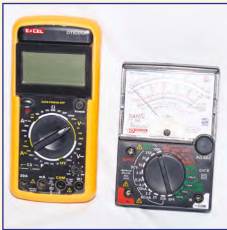
Fig.1. A 20kΩ/V analogue multimeter on the right and a digital type on the left; both offer numerous ranges of voltage, current, and resistance measurement plus transistor and diode testing. The digital unit also has six capacitance ranges
