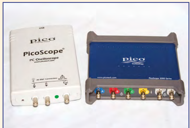
Fig.3. These two units from Pico Technologies enable a PC to be used as a sophisticated oscilloscope. The one on the left is a dual channel type, and the one on the right gives up to four channel operation
