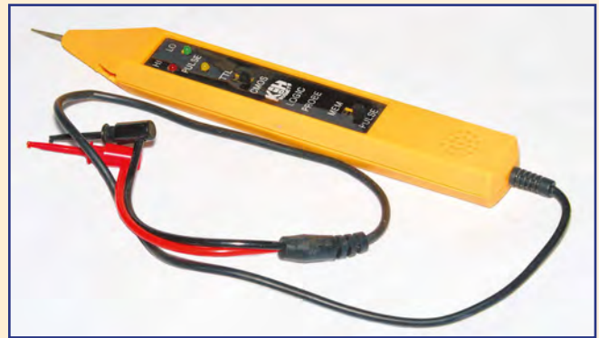
Fig.2. This logic probe can accommodate TTL and CMOS logic levels, and it has LEDs for high, low, and pulsing signals. It has a simple memory facility that enables a single brief pulse to be detected reliably
