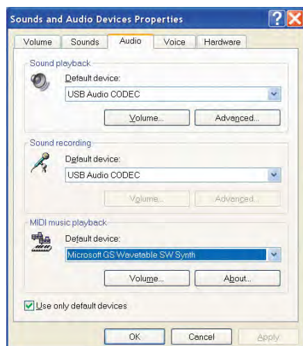
Fig.8: the USB Audio CODEC should become the default device when the USB Stereo Recording and Playback Interface is plugged in (Windows XP dialog boxes).
