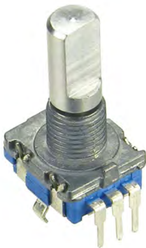
A PCB-mounting continuous incremental encoder with 20 detents per revolution. It uses quadrature output of the encoder to provide direction and pulse. This is typical of the devices used for adjustment controls in domestic appliances
