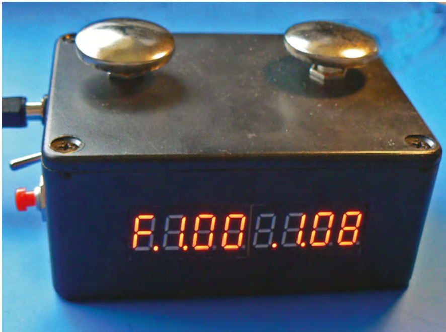
Fig.7. Clock in normal mode – White's flag has dropped after one hour; Black has used eight minutes more
