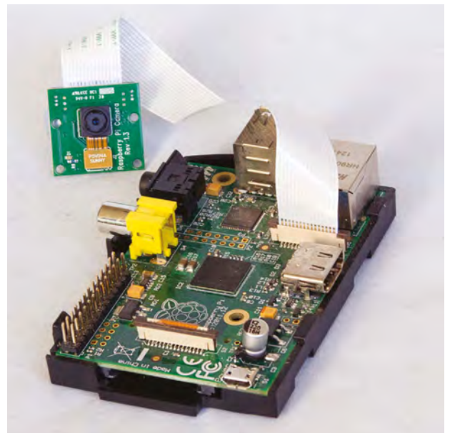
Fig.2. The camera board connected to the CSI port. The maximum resolution for stills is five megapixels, and various video formats can also be accommodated
