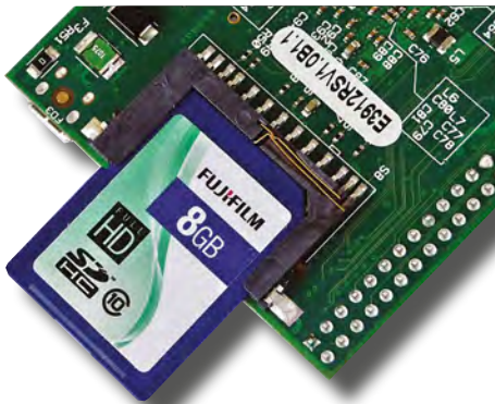
Fig.1.3. An SD card fitted to the slot in the underside of the Raspberry Pi board
