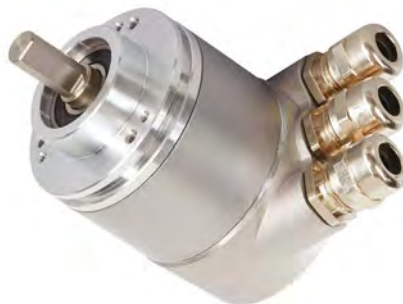
High quality optical absolute multiturn rotary encoder manufactured by FRABA in Germany. This device is protected to IP66 and has resolution of up to 16 bits (65536 steps) per revolution
