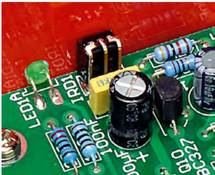
These two photos show the mounting details for the infrared receiver (IRD1). It must be mounted upside down (so that its lens lines up with the adjacent LED), with its leads run down the back of its body.
