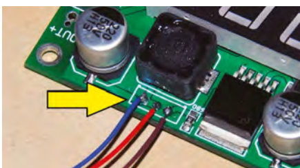
Photo 5: Here are the new leads that run to the remote-mount pot. Solder them on carefully!
