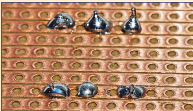
Fig.3. The middle joint in the front row is typical of one where the leadout wire has been cut too short, or is otherwise not protruding far enough through the board. The solder has not flowed over the lead in the bottom right-hand joint
