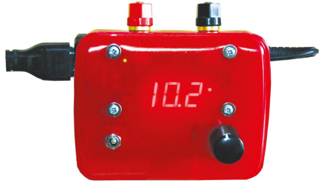
Photo 8: This small power supply features adjustable output voltage from about 1V to 18V, a short-term output of up to 3A, over-current and temperature protection, and an LED display. And it's very cheap to make
