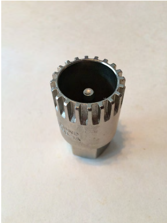
Figure 4-2 You'll need the right tool to remove the bottom bracket
