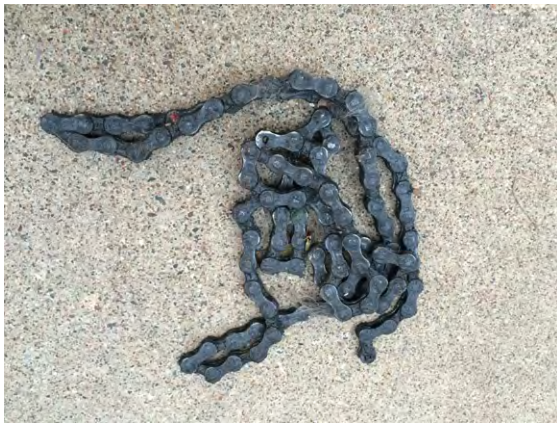
Figure 1-6 A bike chain allows you to turn the rear wheel with the pedals
