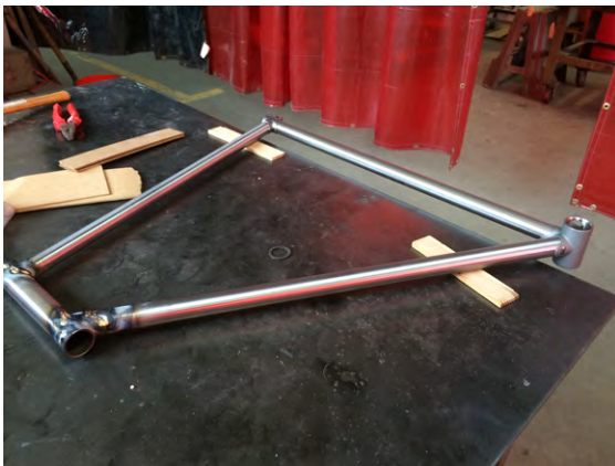
Figure 7-17 Attach the seat tube to the bottom bracket and top tube
