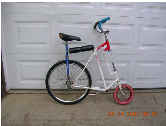
Figure 3-1 A unicycle conversion made from combining two bikes (Photo credit: Peter Wm. Wagner, aka Whymcycles)
