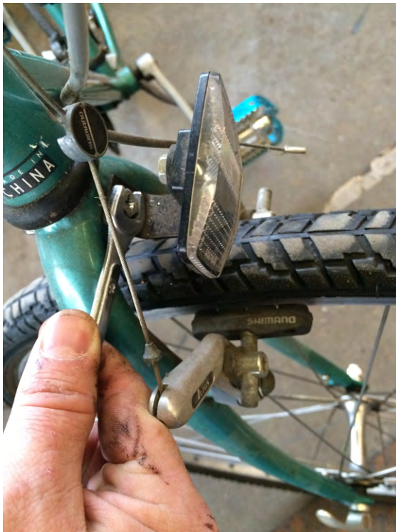
Figure 5-2 Detach the reflectors and other easily removed accessories
