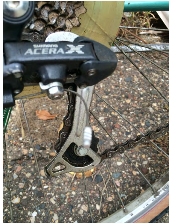
Figure 1-8 Derailleurs control the chains, allowing you to switch speeds while moving
