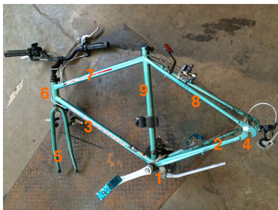
Figure 7-2 Every tube on a bike has a name
