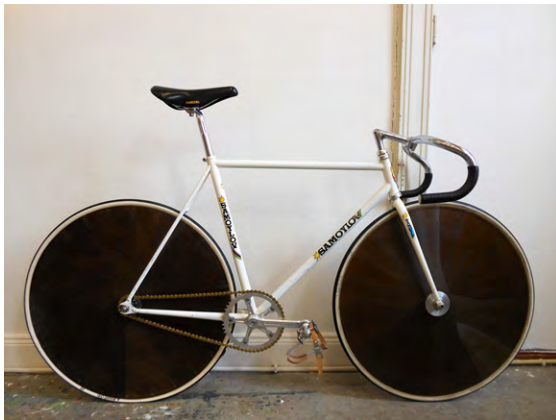
Figure 6-1 This racing bike sports spokeless wheels built out of Kevlar (Photo credit: Sir Braginski)
