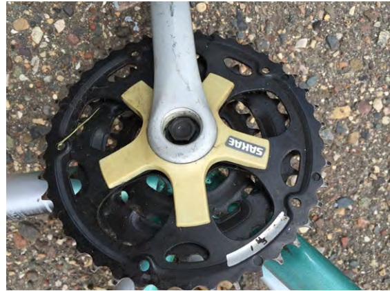
Figure 5-23 Put the chain on the chainring, and either remove or ignore the forward cassette
