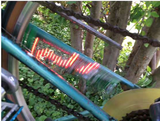
Figure 2-25 A magnet triggers the Hall effect sensor and activates the LED animation
