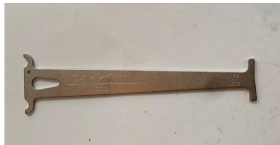
Figure 4-7 The chain wear indicator helps you determine whether to replace your chain
