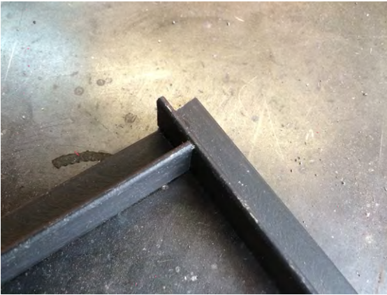
Figure 7-4 Check the fit between the various parts
