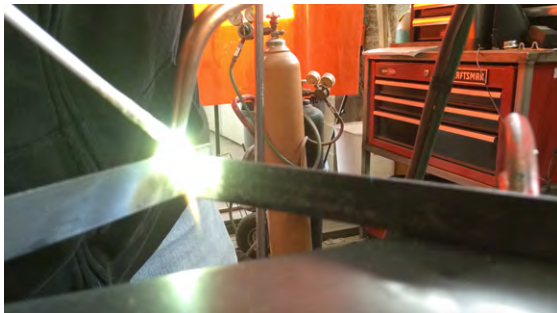
Figure 7-8 Apply braze to the heated joint
