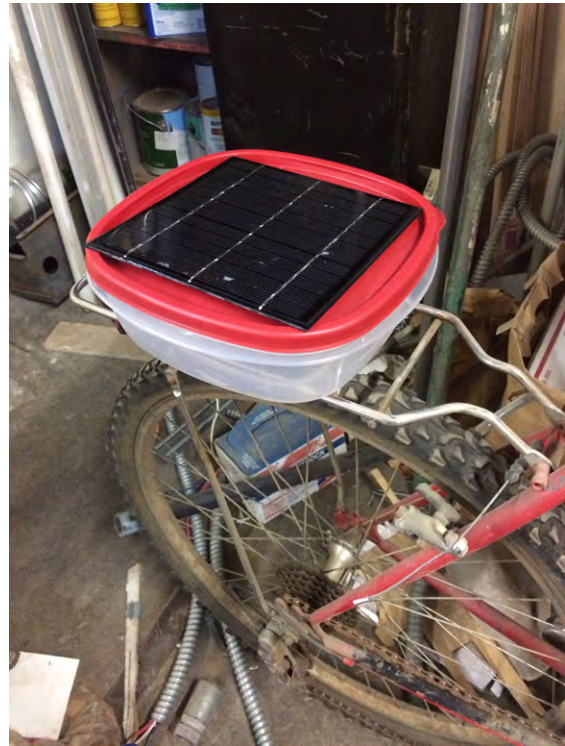
Figure 8-7 Build this solar-powered battery pack
