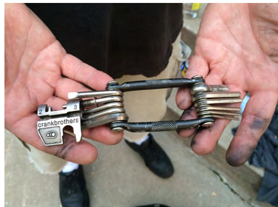
Figure 4-17 Bicycle multitools: more than just a lot of hex wrenches
