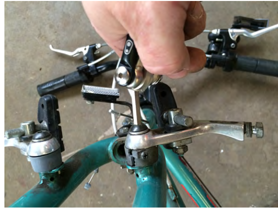
Figure 5-9 Unbolt the brake mechanisms from the frame
