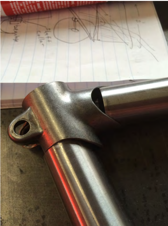
Figure 7-5 Lugs help you join two metal tubes
