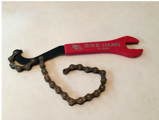
Figure 4-8 A chain whip lets you keep a freewheel-equipped wheel from moving
