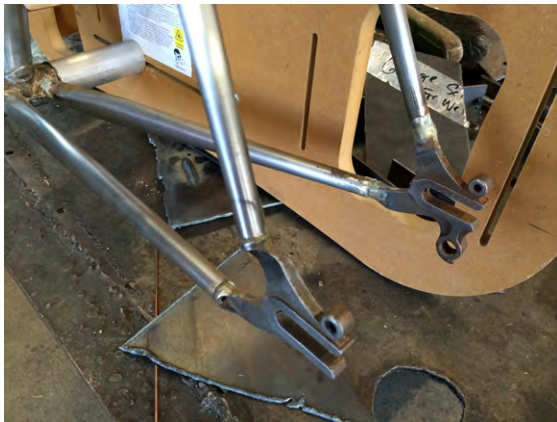
Figure 7-21 Braze on the dropouts
