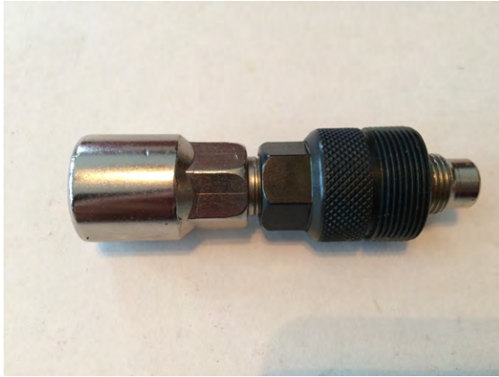
Figure 4-11 Add or remove the cranks with this wrench
