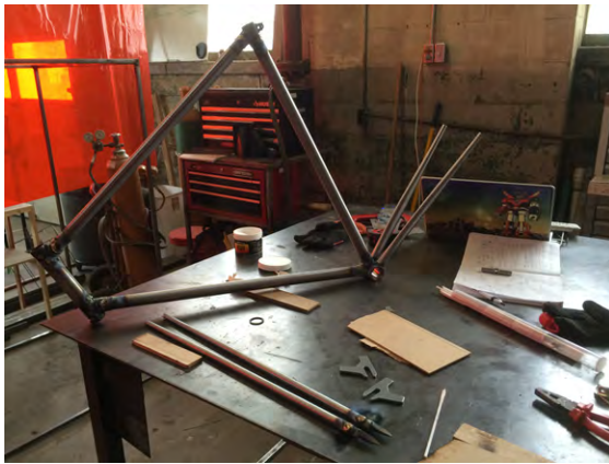
Figure 7-20 Braze the chain stays to the bottom bracket
