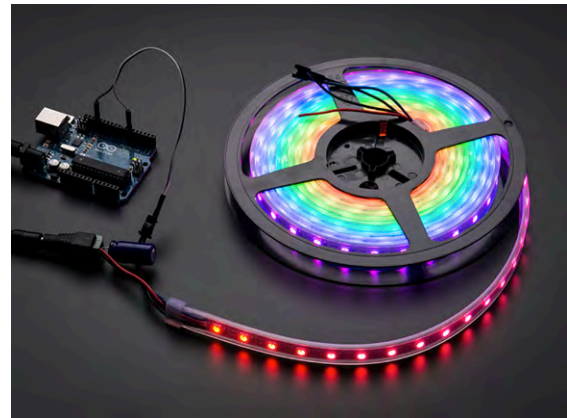
Figure 9-9 NeoPixels are a great line of smart LEDs (Photo credit: Adafruit Industries)
