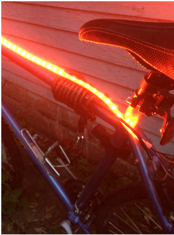
Figure 9-16 Install the light strip on your bike
