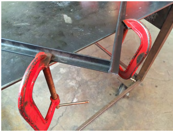
Figure 7-7 Hold the parts in position so they can be brazed
