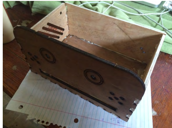
Figure 11-5 Assemble the basket, gluing the seams with regular wood glue
