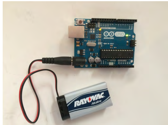
Figure 8-19 Plug the power adapter into the Arduino
