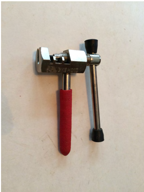
Figure 4-5 The chain breaker is a necessity for working with chain links
