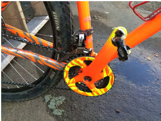
Figure 1-7 Chainrings turn the chain as you pedal
