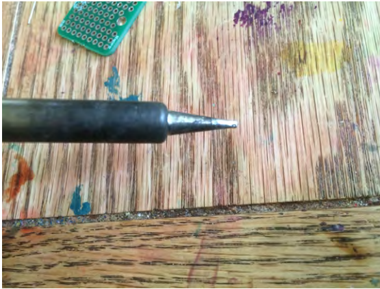
Figure 8-3 Tin the tip of your soldering iron
