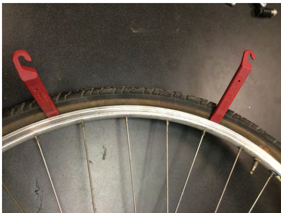
Figure 6-4 Tire levers pull the tire away from the rim
