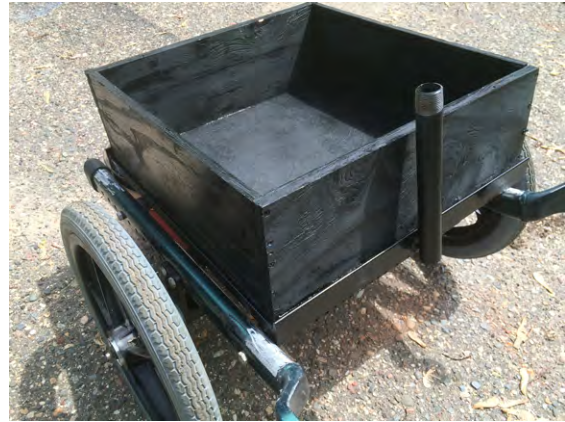
Figure 11-17 Paint the trailer to protect it from the elements
