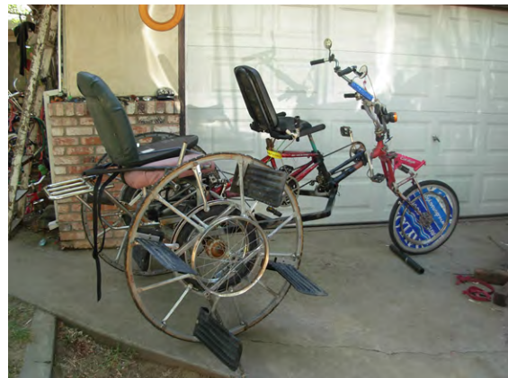
Figure 3-12 This three-wheeled vehicle converts to a paddleboat (Photo credit: Peter Wm. Wagner, aka Whymcycles)
