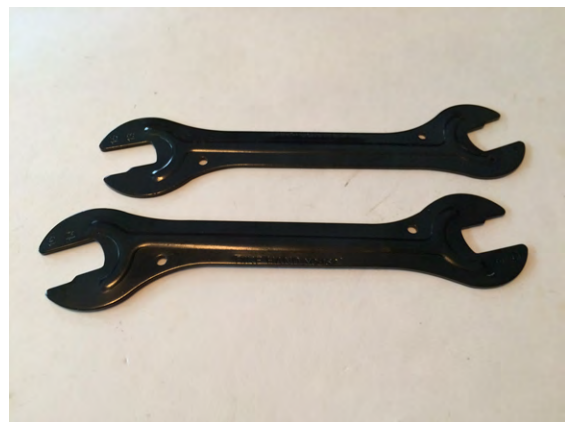
Figure 4-10 Cone wrenches are used to adjust a bike wheel's hub
