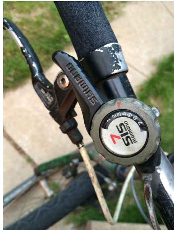
Figure 1-10 Gear shifts control the derailleurs and allow you to move the chain from one gear to the next
