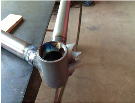
Figure 7-16 Braze up the bottom bracket
