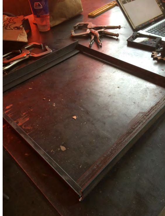
Figure 11-10 Cut lengths of angle iron in order to build your bed
