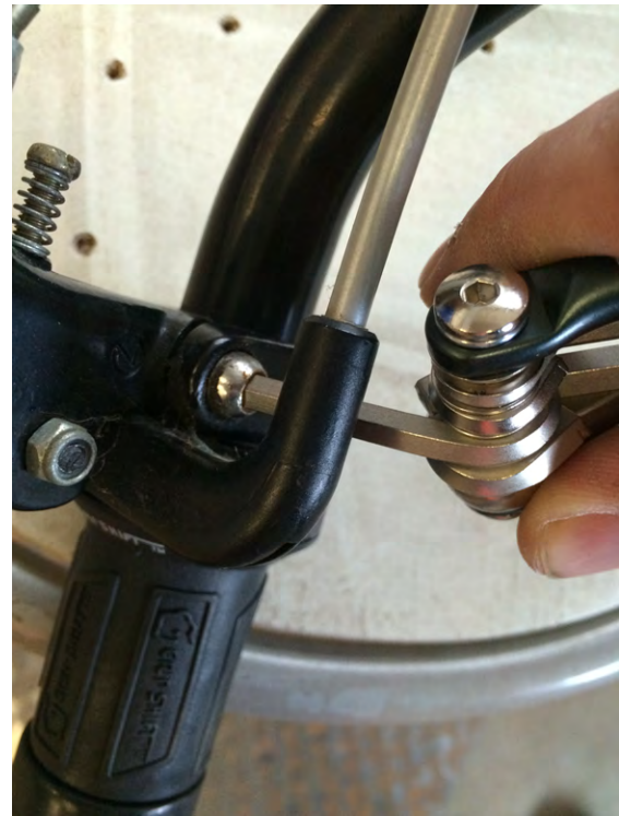
Figure 5-3 Next, remove the gear shifts and brake levers
