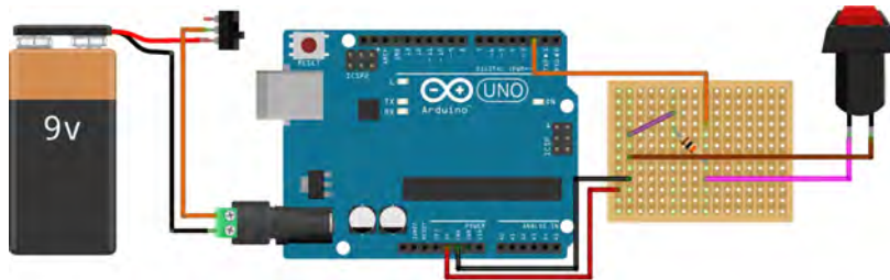
Figure 10-7 Connect the button and its resistor
