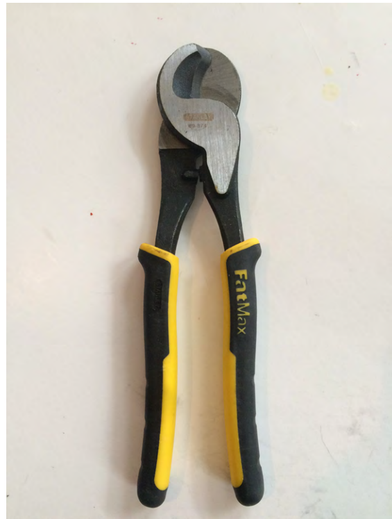
Figure 4-3 A cable cutter helps cut neatly through cables and housings
