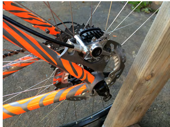
Figure 2-3 Though pricey, disc brakes offer an improvement in braking ability
