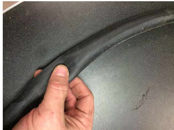
Figure 6-5 Inspect the inner tube for punctures
