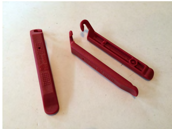
Figure 4-24 Tire levers are a necessity for working on a bike tube
