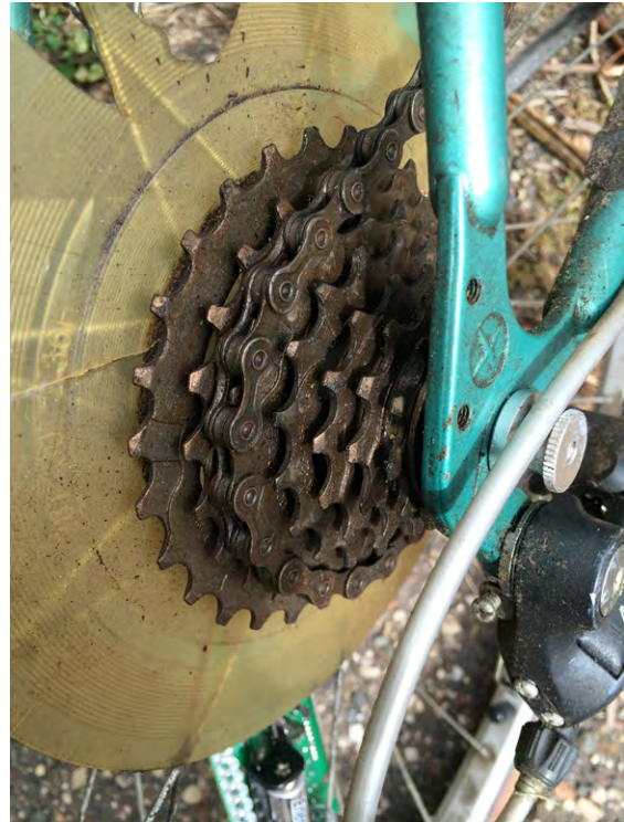
Figure 1-5 The cassette is the stack of gears that the derailleur interacts with
