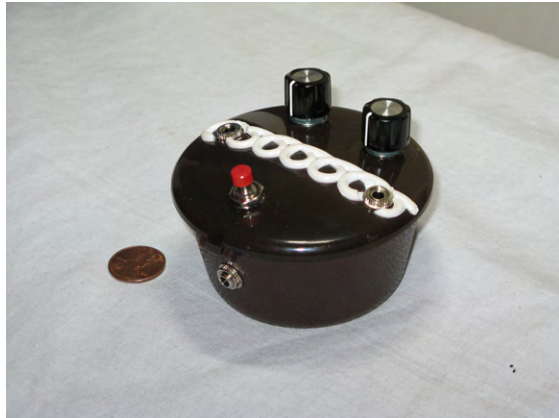
Figure 10-2 The Atari Punk Console is a classic analog noisemaker (Photo credit: Wayne Wylupski, Community Commons)
