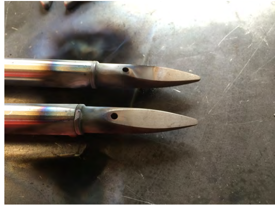
Figure 7-18 Attach two lugs to the seat stays
