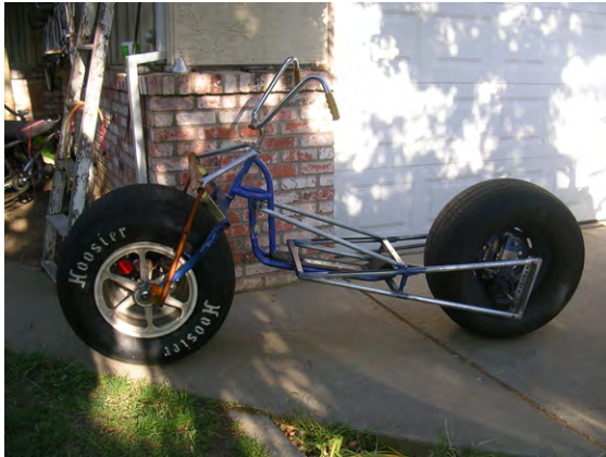
Figure 3-8 Peter Wagner's Whymcycle moves when the rider bounces on it (Photo credit: Peter Wm. Wagner, aka Whymcycles)
