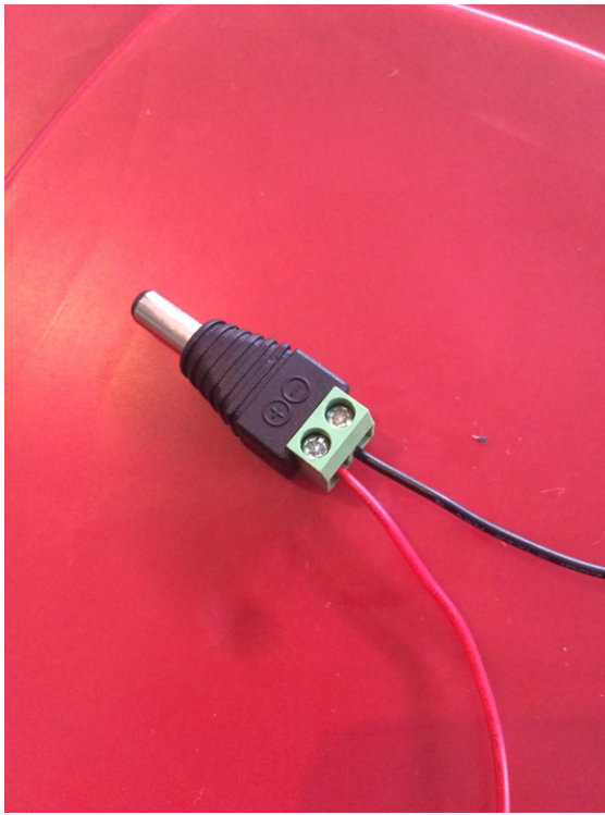
Figure 8-9 Attach the DC power adapter to the solar panel's wires
