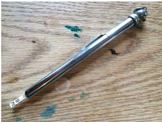
Figure 4-19 Ensure proper wheel inflation with a pressure gauge
