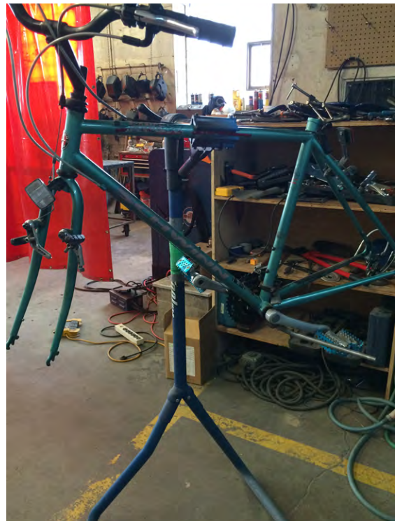
Figure 4-1 The bike stand holds your bike so you don't have to
