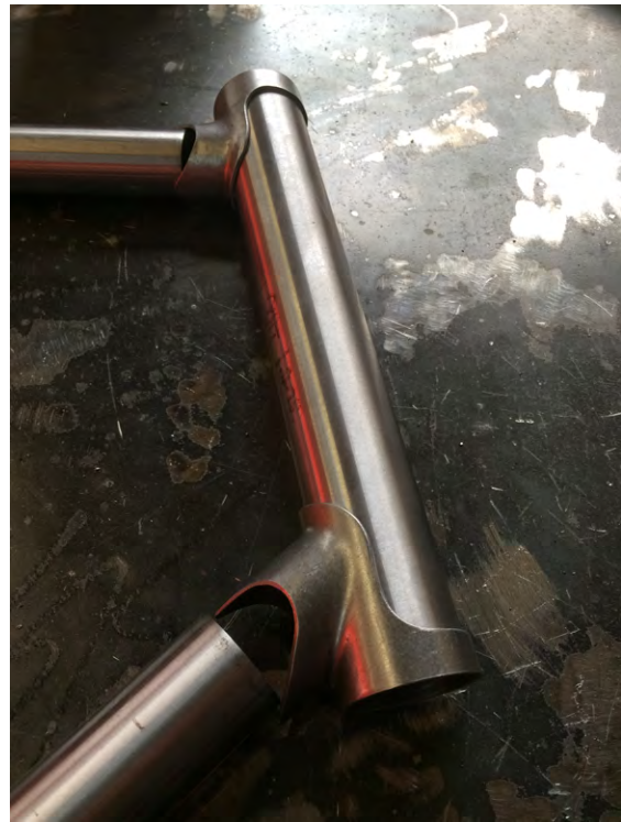
Figure 7-15 Braze the tubes together with the help of some lugs
