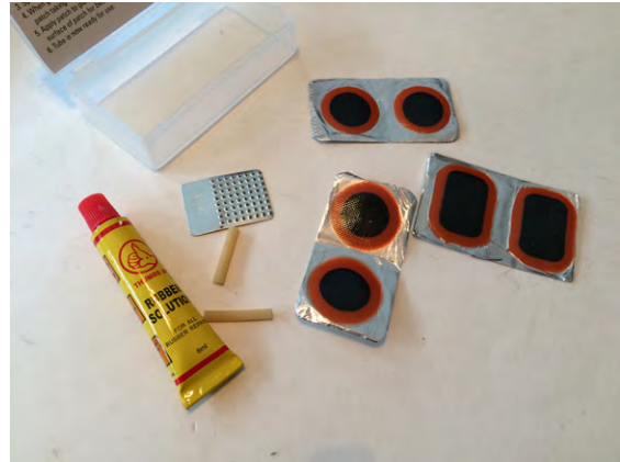
Figure 4-20 Fixing flats requires a rasp and patches
