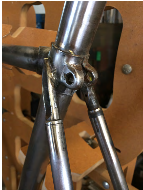
Figure 7-22 Braze the pointy lugs to the seat tube (Photo credit: Gabriel Amadeus, Creative Commons)
