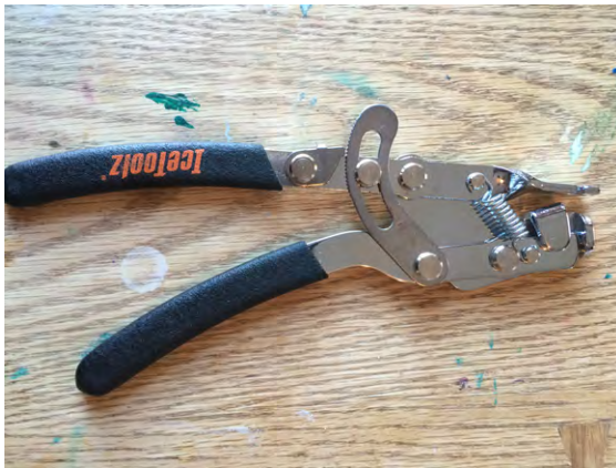
Figure 4-4 The cable puller keeps the cable taut while you secure it
