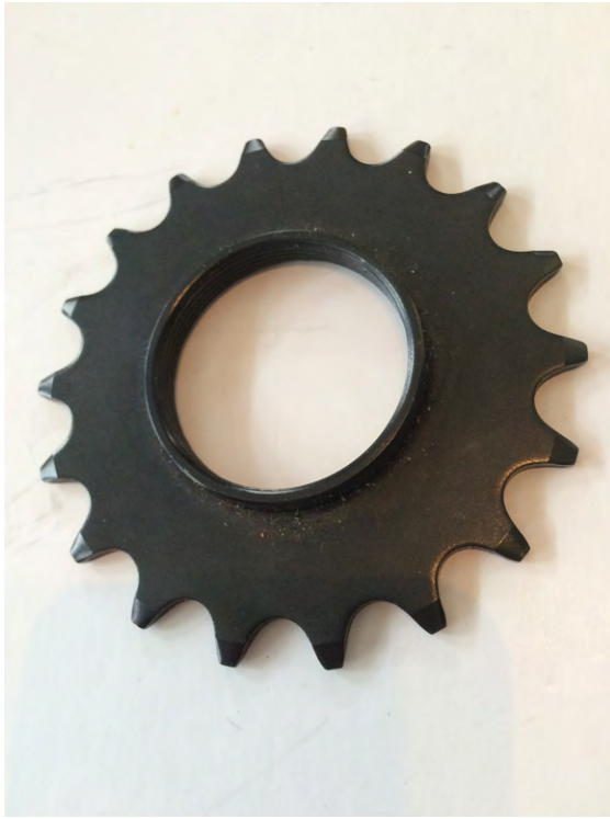
Figure 5-22 A fixie cog takes the place of the gear cassette and freewheel
