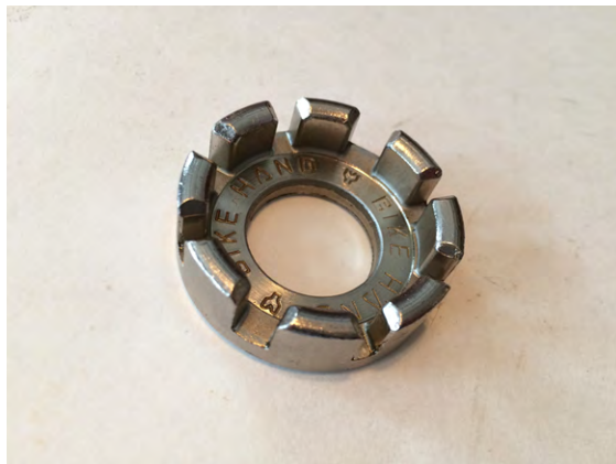
Figure 4-23 A spoke wrench has grooves for various gauges of spoke
