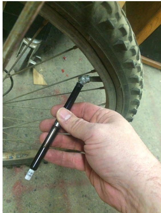
Figure 6-11 Measure the PSI to make sure you're properly inflated
