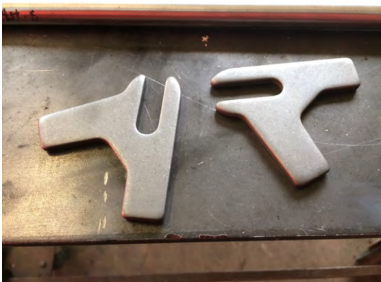
Figure 11-12 Weld on the dropouts
