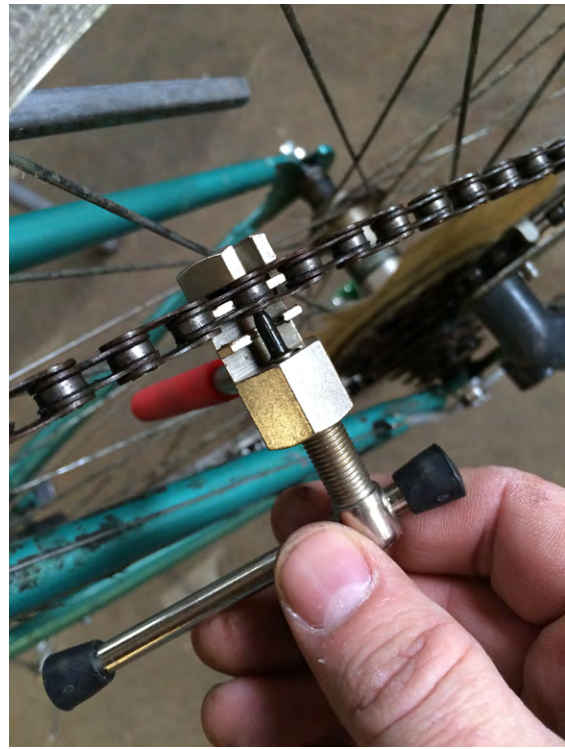
Figure 5-5 Break the chain and remove it
