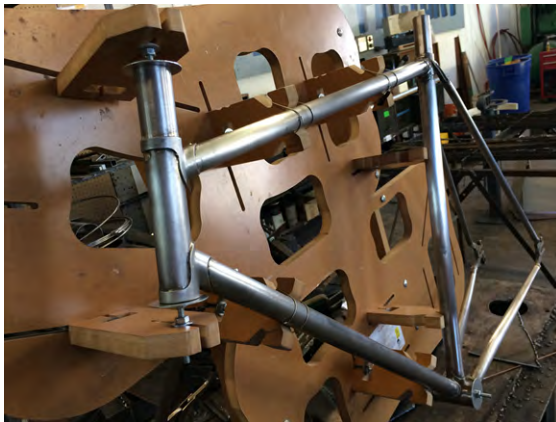
Figure 7-14 Secure the tubes for welding
