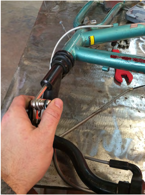
Figure 5-14 Lastly, remove the handlebars and fork
