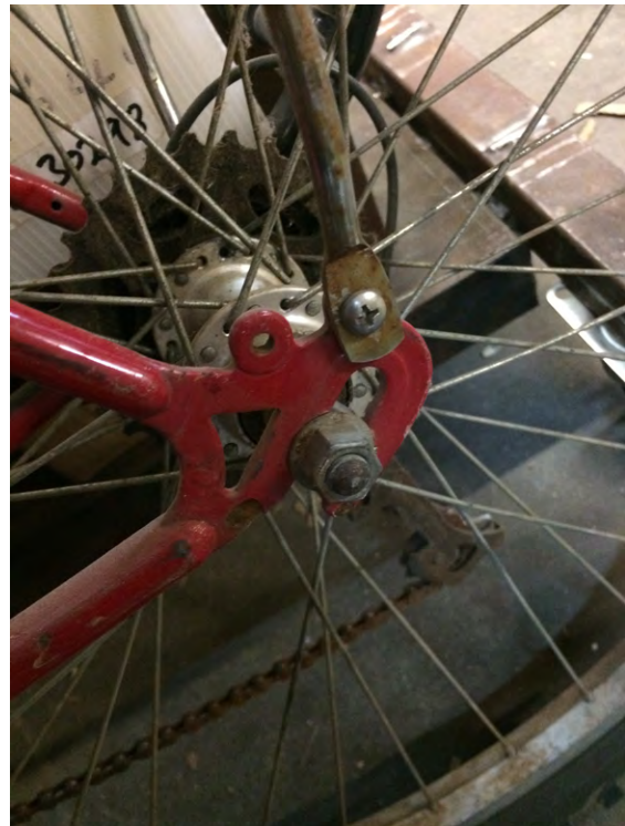
Figure 5-21 Make sure you have this kind of dropout
