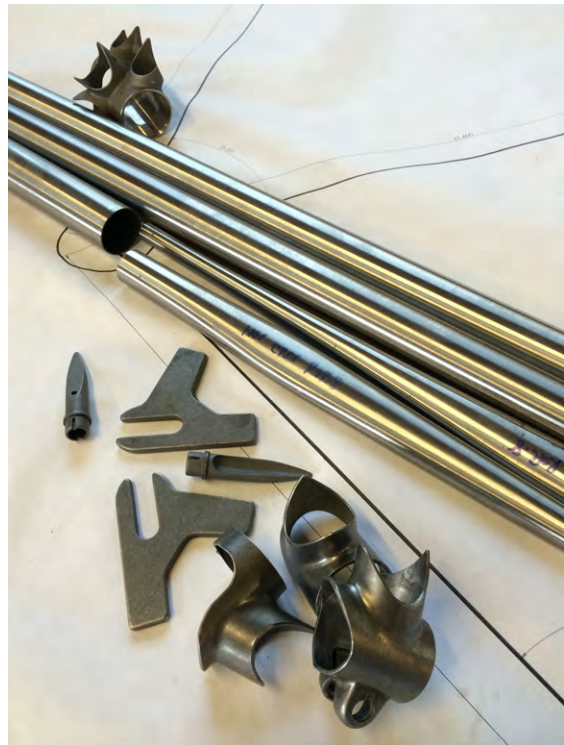
Figure 7-13 Cut the tubes so they fit together
