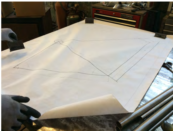
Figure 7-11 Design your frame at 1:1 scale
