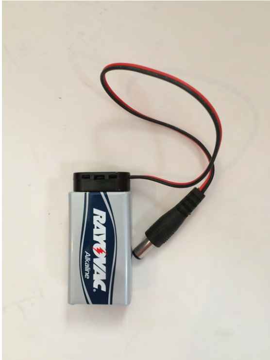
Figure 8-18 The battery plugs into the cable
