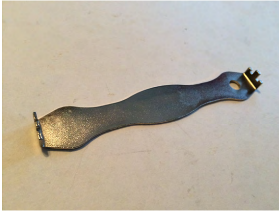
Figure 4-18 Secure your pedals using a pedal wrench
