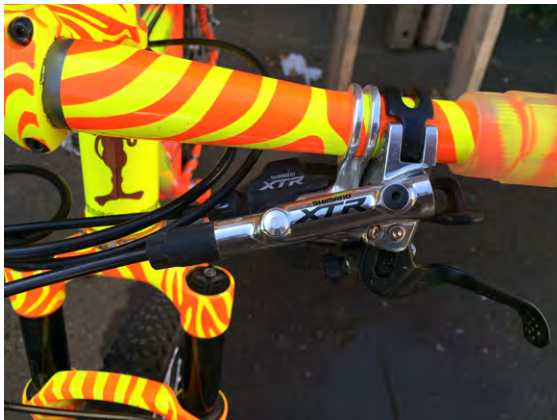
Figure 1-4 Squeeze the lever to slow down the bike
