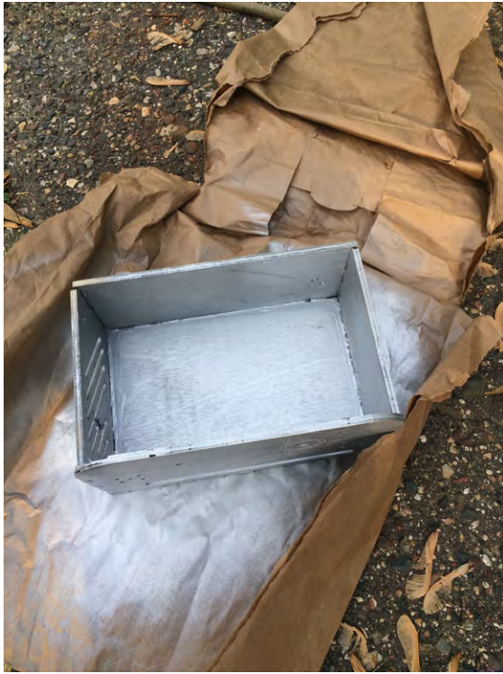
Figure 11-6 A couple coats of spray paint will make the basket last longer
