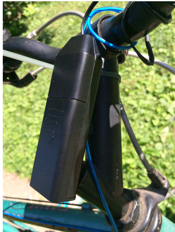
Figure 2-20 Zip-tie the inverter
