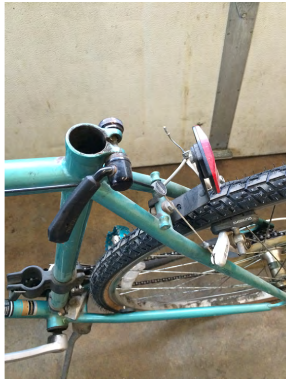
Figure 5-1 Remove the saddle
