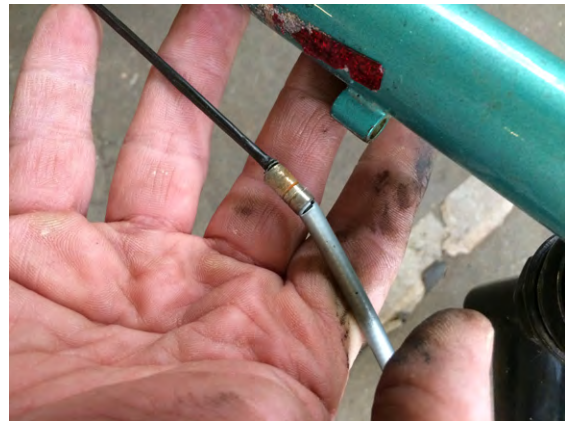
Figure 5-10 I found lots of damage when I removed the cables
