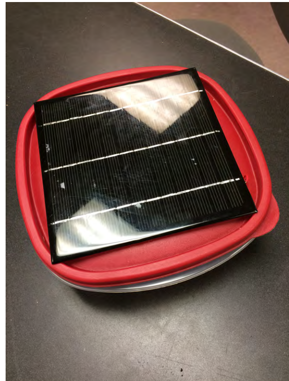
Figure 8-15 Attach the solar panel to the lid of the box
