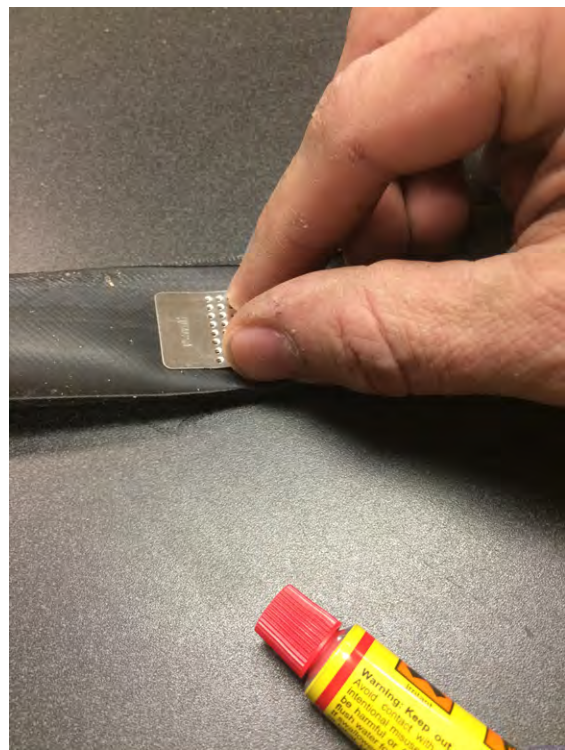
Figure 6-6 Roughen the area around the puncture
