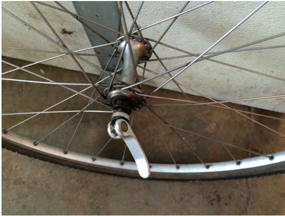
Figure 5-7 The front wheel has a quick-release to help you remove it rapidly
