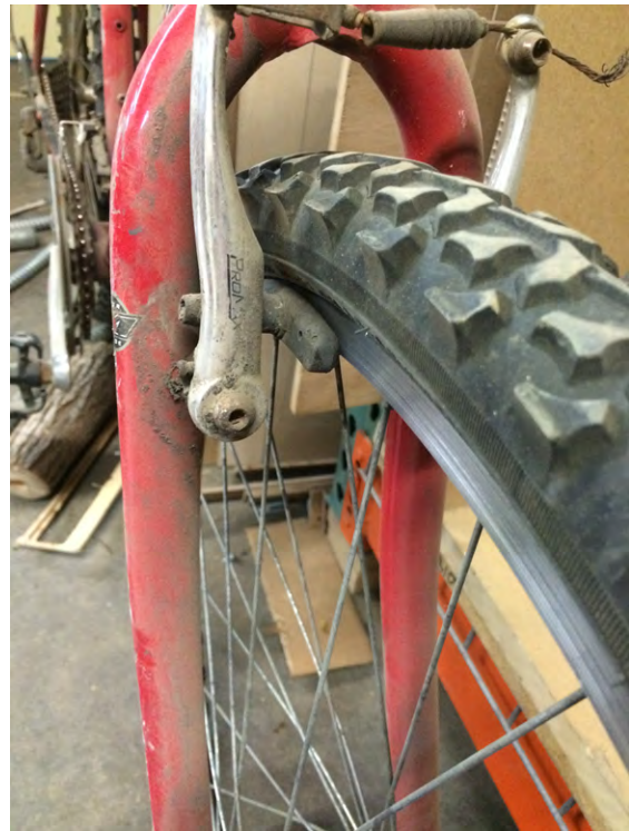
Figure 6-13 Watch the space between the rim and the brake pad
