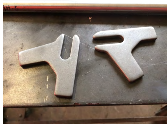
Figure 7-19 Cut slits in the stays to accommodate the dropouts
