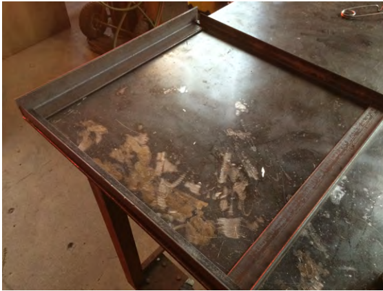
Figure 11-11 Weld or braze the trailer's frame
