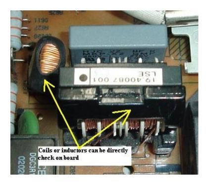
Inductor or coil testing can be done on board without removing the coil out from the circuit board. If a coil has less loops (small coil), then we can just direct measure it with our normal ohmmeter. A small coil is just like a wire or a jumper and it rarely become defective although it has some inductance value in it. Testing coils that have a bigger inductance value like the B+ coil used in Monitor circuit is different from checking the small coils.
