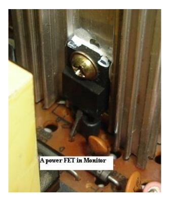
Many switch mode power supply are using the combination of a power FET and a PWM IC design to switch the power transformer. Whenever there is any power failure (fuse totally blown into dark colour) one will always suspect the power FET has gave way. Usually we would use the black probe set to X 1 ohms and place it to the centre pin (drain) and the red probe to the gate and the source pin.
