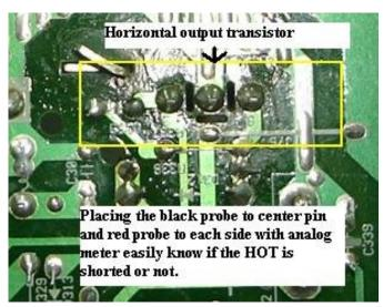
Checking horizontal output transistor is so easy and you can check it on board. Set your analogue meter to X 1 ohm and place the black probe to the centre pin (collector) of the HOT and the red probe to base and emitter. It should not register any reading. If there is a reading, most probably the HOT has developed a short circuit.
