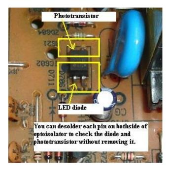
Optoisolator or optocoupler IC's usually located in between the primary and secondary side of power supply and can be test even if the IC is still on board (you can actually test this type of IC with your multimeter). Some of the famous optocoupler part numbers are 4N25, 4N35, PC123 and etc. Just desolder one pin on each side (assuming this optocoupler have 2 pins on each side) of the optocoupler. Pin 1 and 2 is the LED light and pin 3 and 4 is the phototransistor collector and emitter.
