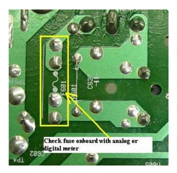
Next is the fuse, you can easily check it on board with your multimeter. Just set your meter either to ohms or continuity. A good fuse should have reading (ohms value) and beep sound if you select the continuity test. If no reading or sound, 100 % the fuse is open and need replacement. Replace only with the same ampere and voltage rating of fuse.
