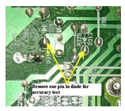
In order to accurately check diodes, you need to desolder one lead and test it with an analog meter set to X 10k ohms range. A good diode should have only one reading while the bad one will have two readings. Be careful if you want to test a Schottky diodes as Schottky diodes will have two readings but not shorted readings. If you get two similar readings then the Schottky diodes is considered bad.
