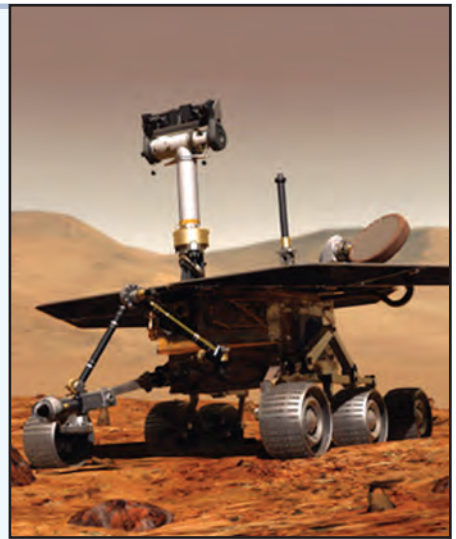
Solar panels supply the electricity used by this "rover" as it explores the planet Mars.
