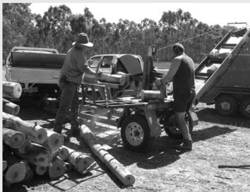
Figure 11.6: Traditional sawbench, loading the billets onto the bobcat's forks. The pile of billets is ready for cross-cutting, splitting and loading.
