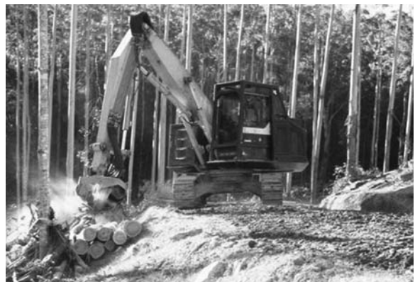
Figure 9.10: Mechanical harvesting is efficient and safe but contractors usually require large volumes and good access.
