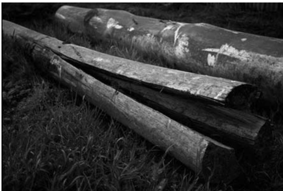
Figure 9.5: Radial splitting in this small-diameter eucalypt log illustrates the difficulty of sawing quarter-sawn boards from small-diameter logs.
