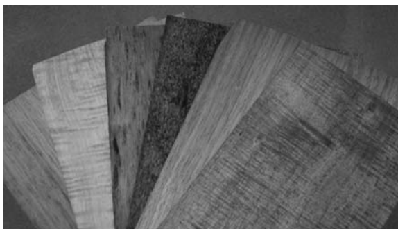
Figure 10.2: Sliced veneers of Australian blackwood ( Acacia melanoxylon ) show a range of colour and grain patterns.
