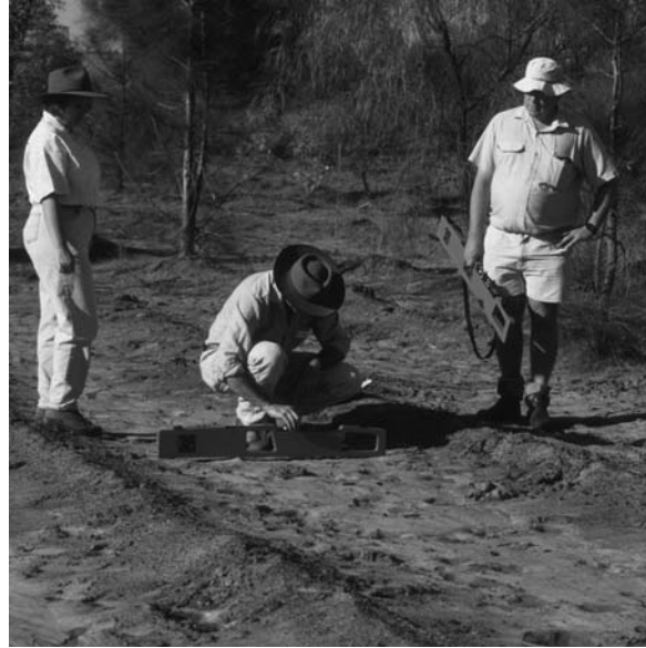
Figure 15.4: Assessment of soil electrical conductivity near Wellington, New South Wales, by electromagnetic induction using an EM38 meter (photo by Nico Marcar).
