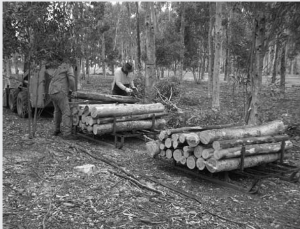
Figure 11.7: Sled system: billets tied to sleds and being cross-cut by powerful chainsaws with long bars.
