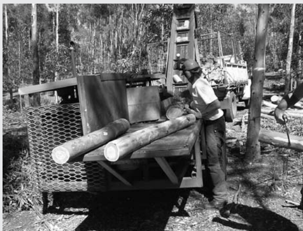
Figure 11.8: 'At stump' system: billets being cross-cut and loaded into the tiptruck by the elevator.
