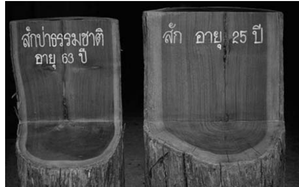
Figure 9.17: The width of the sapwood band reflects the vigour of the tree canopy. The teak tree ( Tectona grandis ) on the left was from a 63-year-old high-stocked plantation in northern Thailand, and the other was from a widely spaced 25-year-old plantation in the same area.
