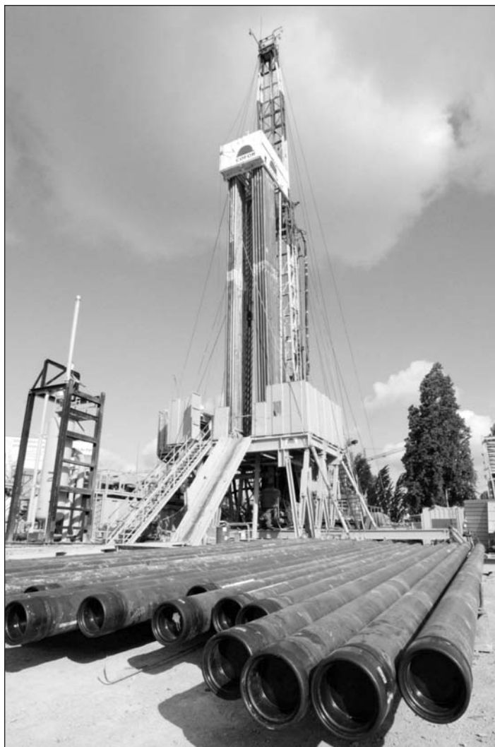
A geothermal drilling rig in Paris, France, participates in an initiative to provide clean heat for the entire nineteenth arrondissement. (Benoit Tessier/Reuters/Landov)
