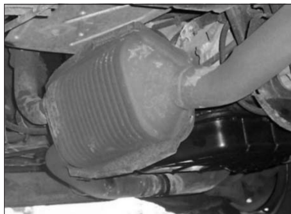
A catalytic converter on a 1996 Dodge Ram.
