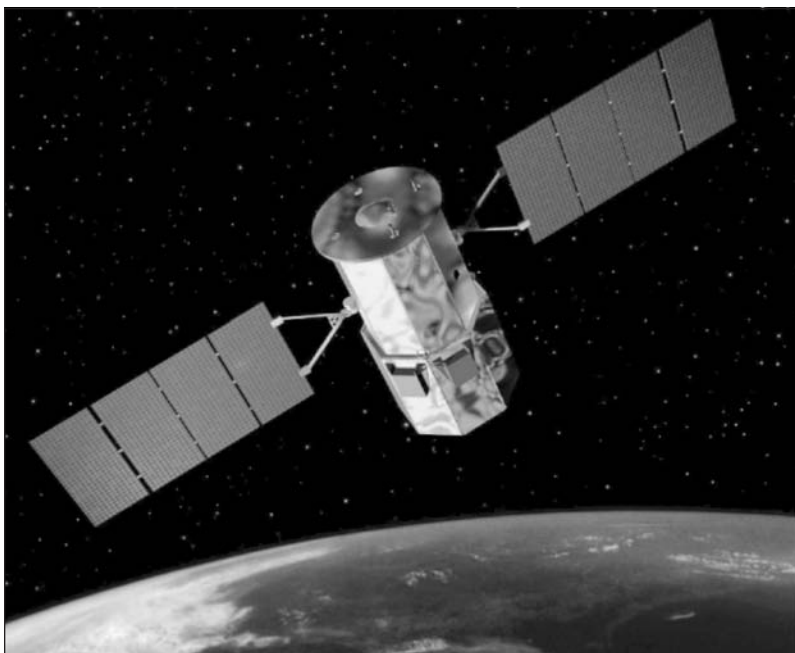
An artist’s rendering of the satellite Glory, which measures the effects of noctilucent and other clouds, as well as those of particles and solar energy, upon climate change. (MCT/Landov)
