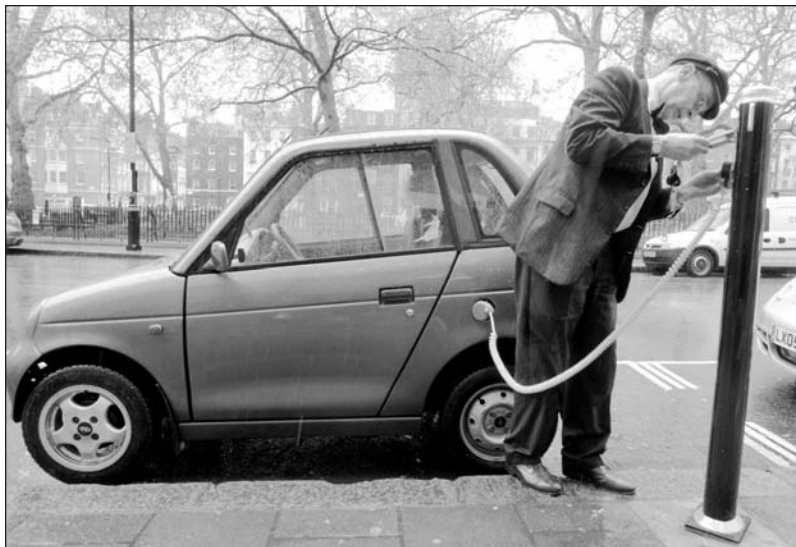
Some hybrid automobiles are capable of recharging their batteries by plugging into charging stations such as this one in Berkeley Square, London. (Getty Images)
