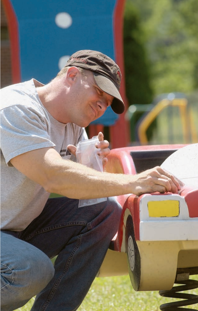
An air quality engineer scrapes soot from playground equipment. The sample will be sent to a lab for testing. AP Photo/Beaver County Times/Sally Maxson
