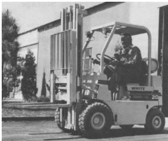
Figure 1. Common forklift, useful for moving batches of stored cones as well as numerous other nursery containers.
