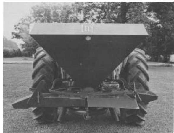
Figure 12. Broadcast seeder may be used to spread granular (solid) chemical fertilizer.
