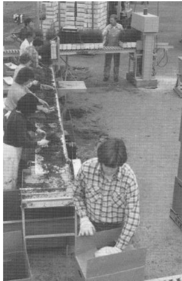
Figure 6. Assembly-line operation: plugs are loosened with an extractor, removed from their containers, and then packaged for shipping.
