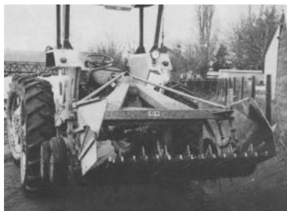
Figure 19. Seedling lifters loosen soil so that seedlings can be manually extracted.
