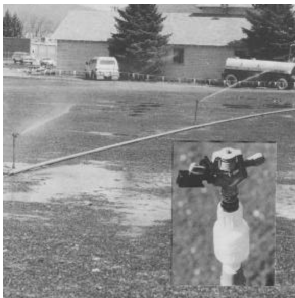
Figure 10. Impulse sprinkler systems (sprinkler head shown in inset) have adjustable water trajectories and rotation patterns.
