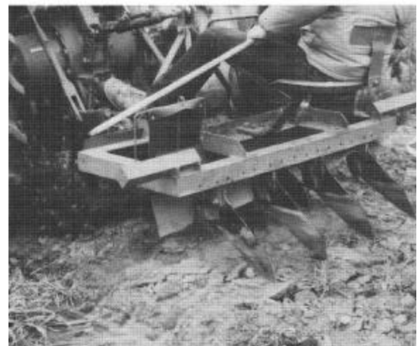
Figure 9. Lateral root pruning between the drill rows to sever excessively long lateral roots.
