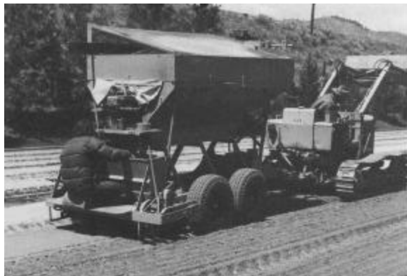
Figure 13. Sand spreader useful for adding mulches to soil.
