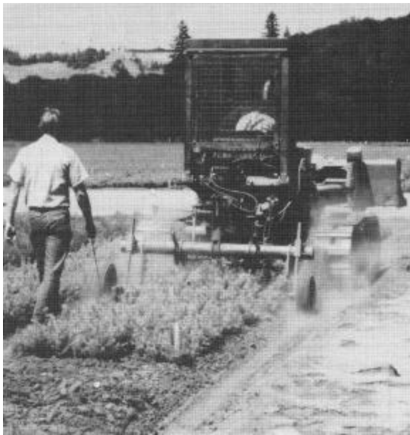
Figure 8. Root wrenching 2+0 Douglas-fir seedlings with a fixed blade tilted at a 20 to 30° angle.
