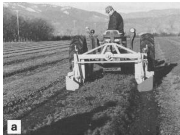
Figure 15. (a) Budding wheel hoe row cultivator and (b) Coeur d'Alene path cultivator keep nursery beds weed free.
