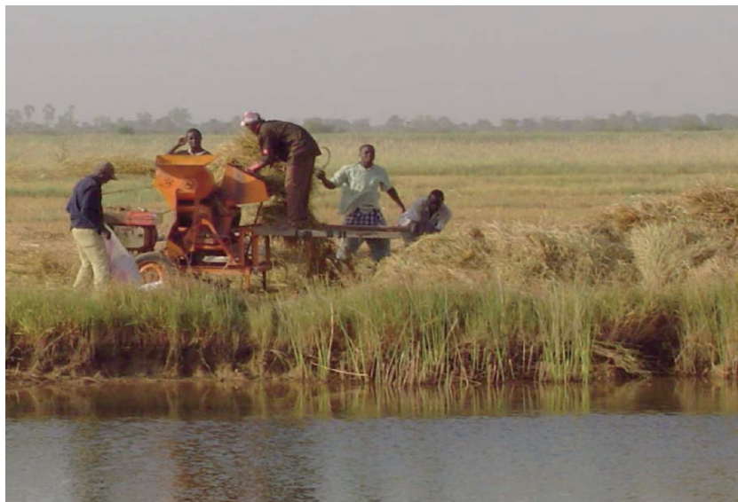
Figure 10-2. Small rice threshing unit in operation in the Office du Niger, Mali. (Reproduced by permission of Dr Frans Geilfus and CDP, Utrecht.)
