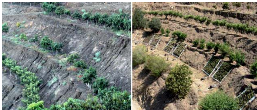
Fig. 8 Gullies in the taluses of orchard terraces and plots used for monitoring the erosion control by plant covers
