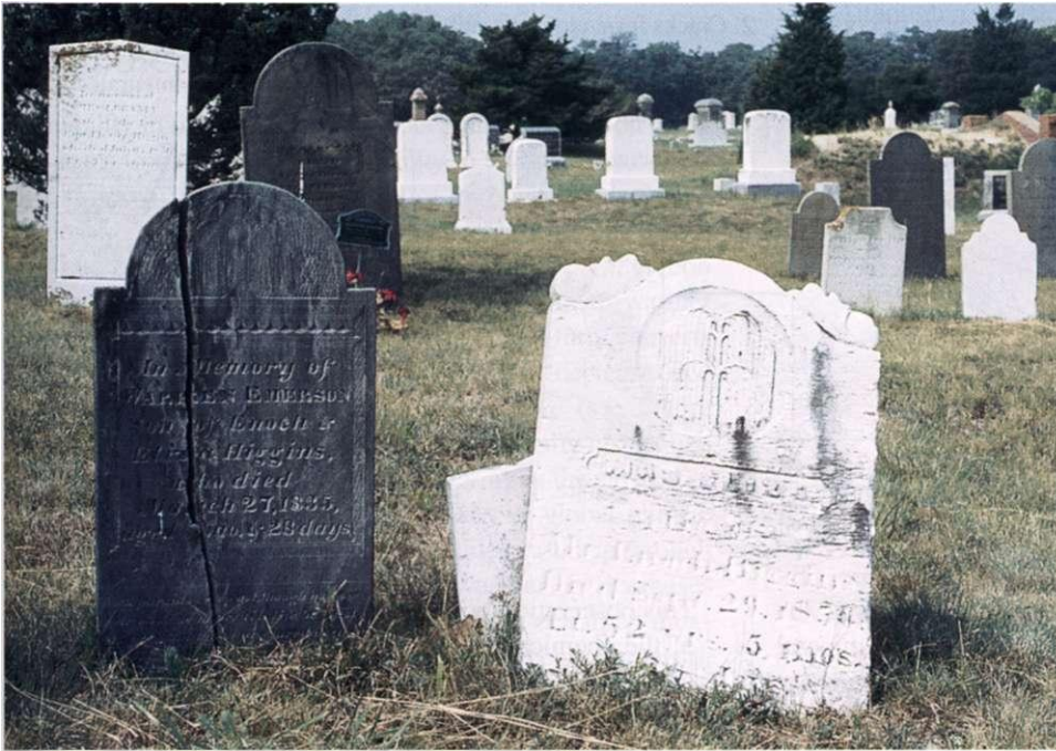
Figure 16.1 Early-nineteenth-century gravestones at Wellfleet, Massachusetts. The stone on the right is limestone and is so weathered that it is unreadable. The stone on the left is slate, which retains its legibility under the same conditions. [Courtesy of Raymond Siever.]
