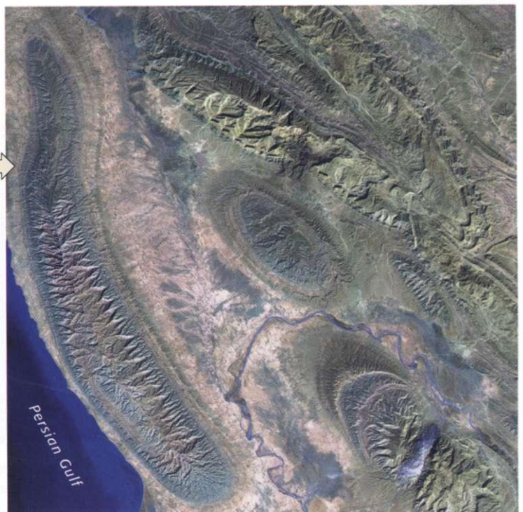
Figure 22.9 Valley and ridge topography formed on a folded terrain of sedimentary rock. The deformation is so recent (Pliocene) that erosion has not yet significantly modified the original structural forms of anticlines (ridges) and synclines (valleys). Zagros Mountains, Iran. [NASA.]
