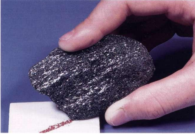
Figure 3.18 Hematite may be black, red, or brown, but it always leaves a reddish brown streak when scratched along a ceramic plate. [Breck P. Kent.]
