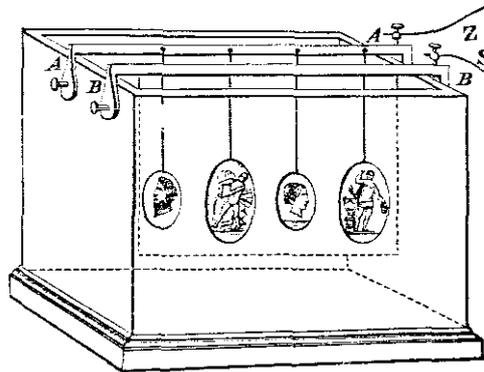
be electrotyped, suspended from the bar *A A*, may be visible; they are supposed to be *behind* and *closely facing* the copper plate. The bar *A A* is connected by the wire *Z* to the zinc pole of the battery.
