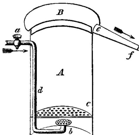
and issuing from *b*, passes through the material, becomes loaded with the volatile matter, rises into the capital, condenses, and passes through *f*, into a worm or other suitable condenser.
