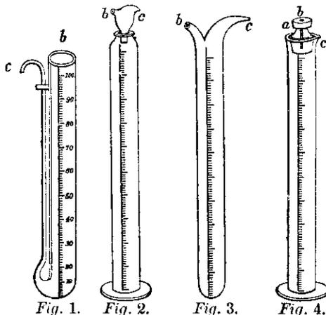
the contained liquid; *b*, the orifice for the ingress of air, to be stopped by the finger or thumb; in Fig. 2, both orifices are in a hollow movable stopper; in Fig. 4, the air-hole only is in the stopper, *a*.
