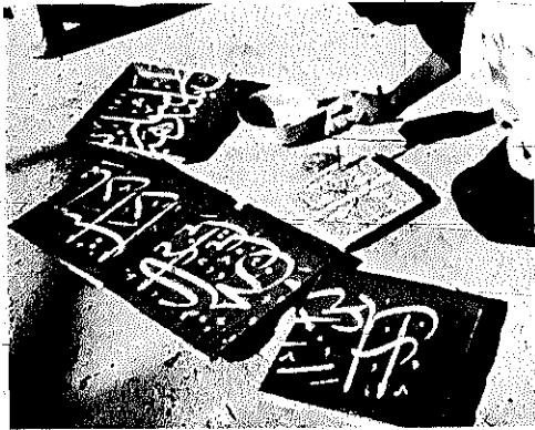
Figure 247—Applying Decorating Glaze
