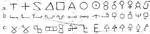
Figure 200 Stonemason's Marks. (a) Found in Persepolis (fifth century B.C.) and on Safavid buildings of the seventeenth century A.D., (b) and (c) Found on the latter only.
