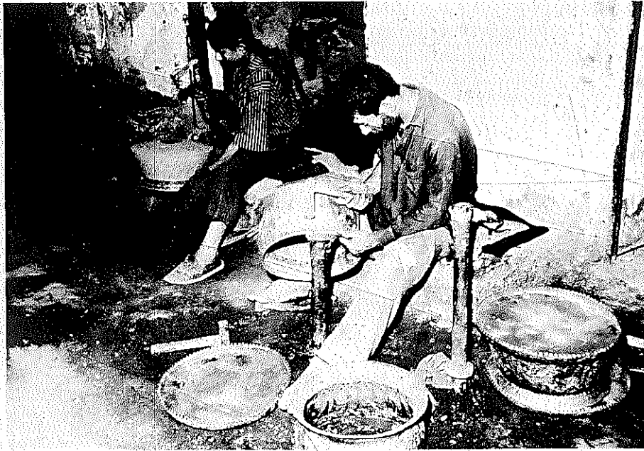
Figure 27 Coppersmiths Planishing (left) and Flanging (right)
