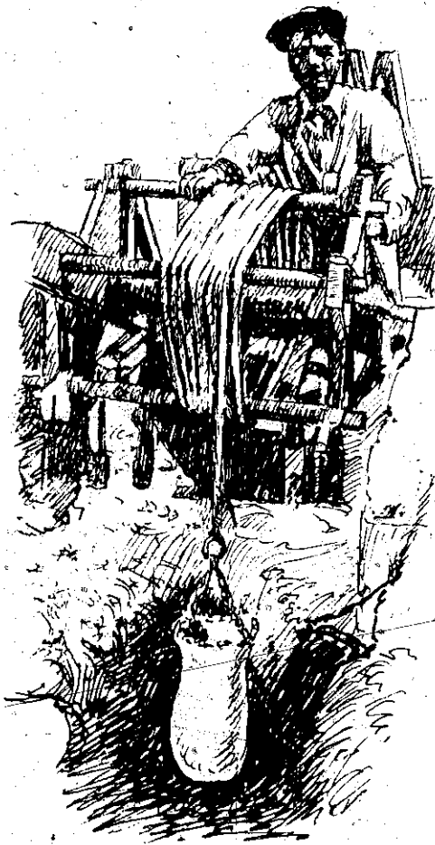
Figure 343. A Household Well with Windlass
