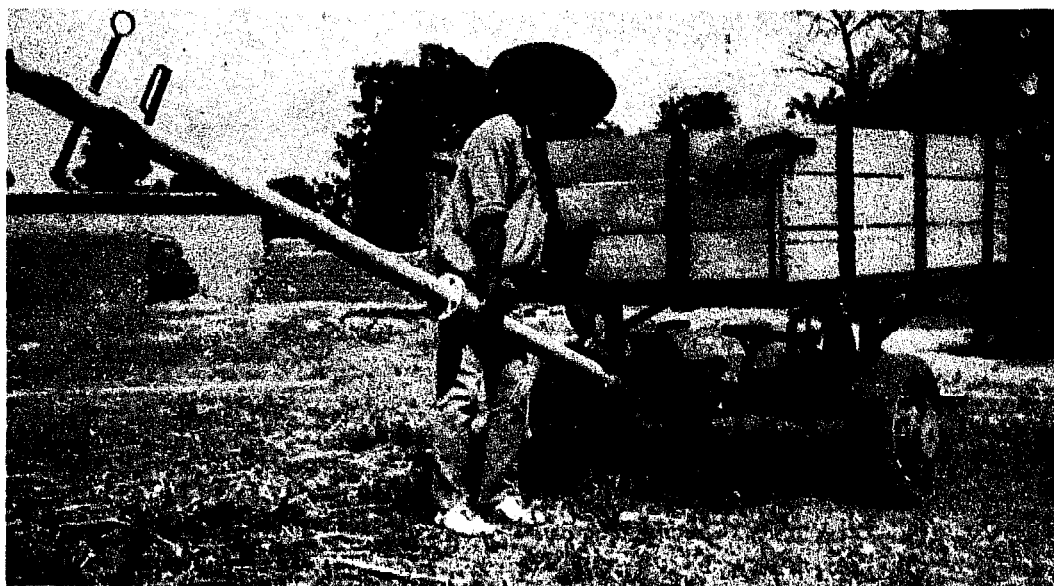
Fig. 8-24: A cart-body on a "Nikart" wheeled toolcarrier in Mali. The farmer found his normal cart more satisfactory and stopped using the toolcarrier altogether. Although toolcarriers have been used as carts, they have seldom been as good as purpose-built carts. Photo: Paul Starkey
