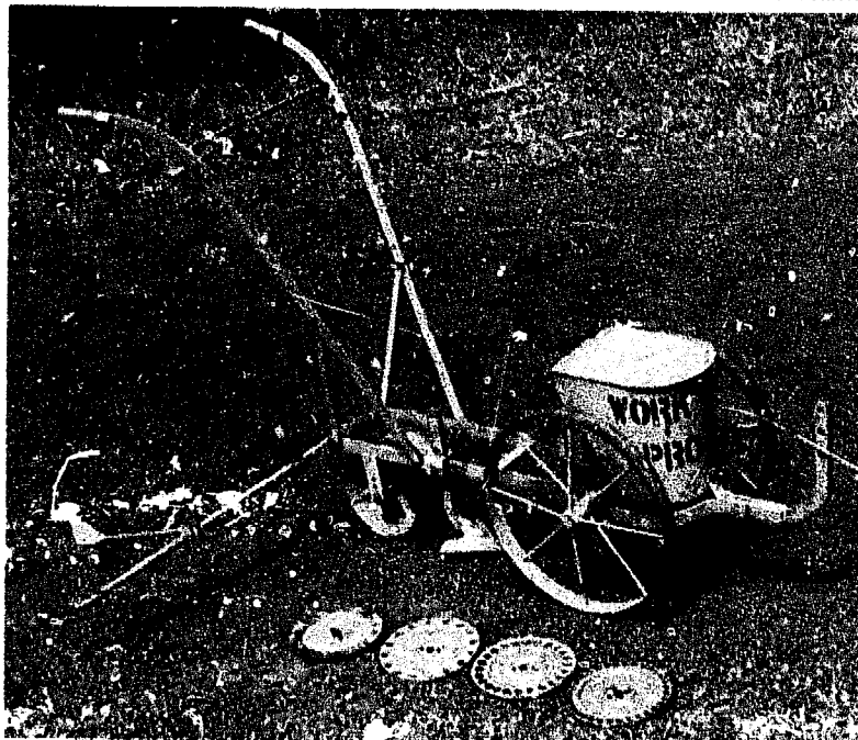
Fig. 7-31: Super Eco seeder. Below: Seeder with various distribution plates and next-row marker extended. Right: Seeder in action showing back of distribution plate and seeds falling into seed tube. The furrow opener, press wheel and row marker are just distinguishable. The ground wheels turn a sealed gear mechanism that drives the distribution plate.
