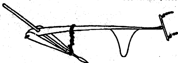
Fig. 7-8: A modified maresha ard. It was developed in Ethiopia by the International Livestock Centre for Africa (ILCA) to allow use by a single animal. The beam was shortened and a skid and swingle tree were fitted. On-station trials were encouraging, but farmer uptake has been low.
