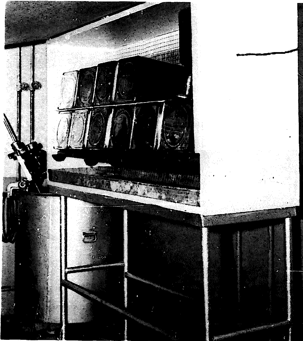
A dry heat cabinet will liquefy 60 pound cans of granulated honey for repacking. — University of Guelph Photo.
