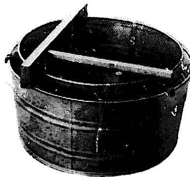
Uncapping can. This separates the free honey from the cappings as they fall from the uncapping knife. The cappings are held in the perforated basket while the free honey drains into the tub below.
