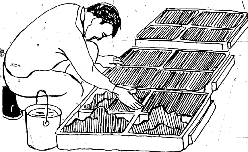
Figure 40. Kneading and leveling the blocks.
