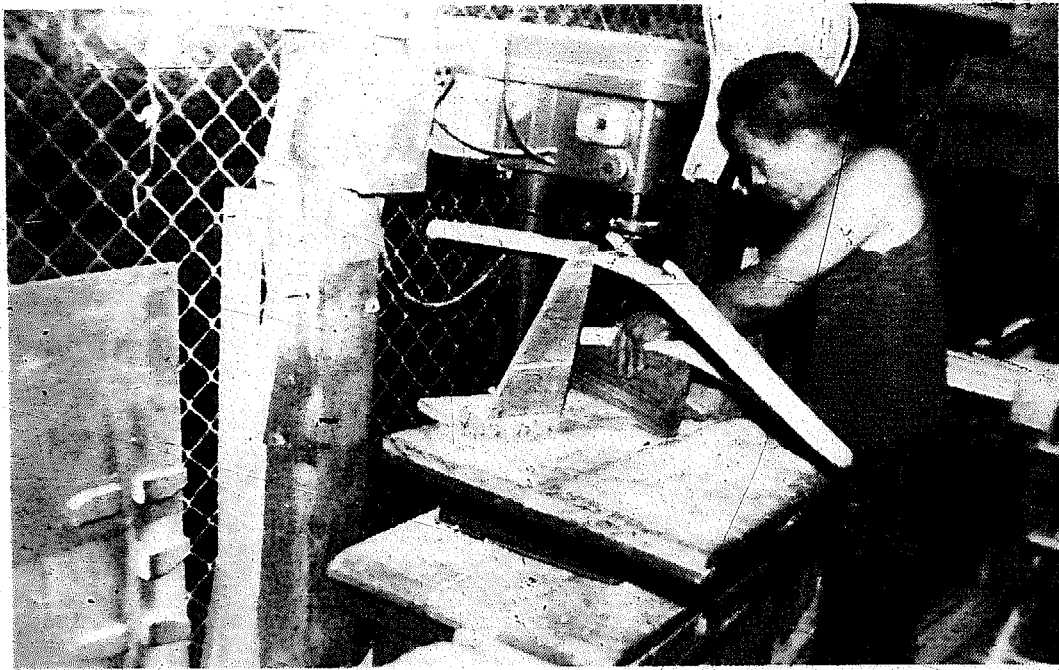
Figure 43. Drilling a chair back leg to take stretcher rail
