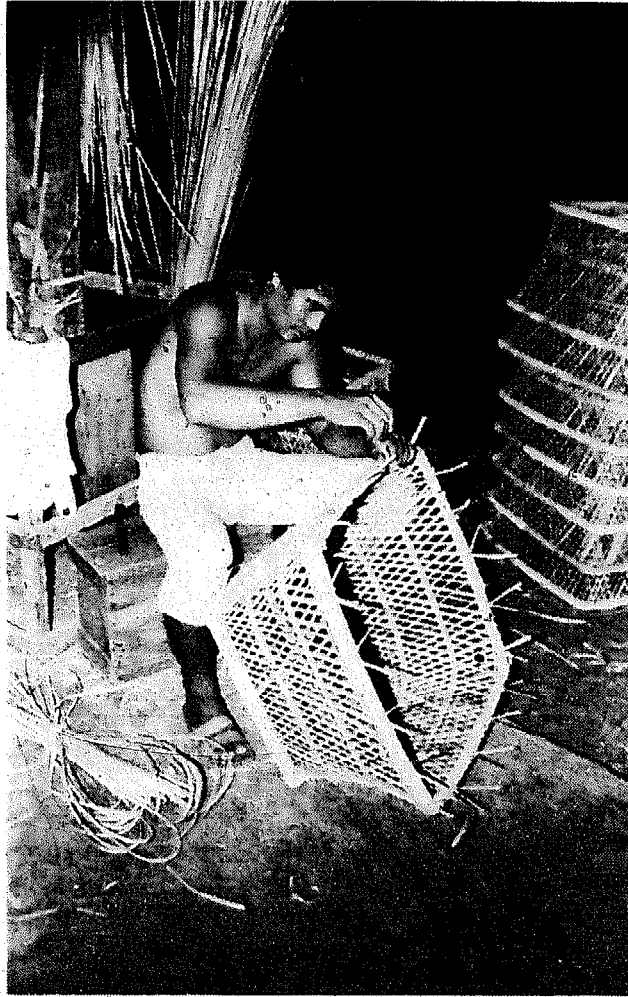
Figure 59. Weaving with rattan peel
