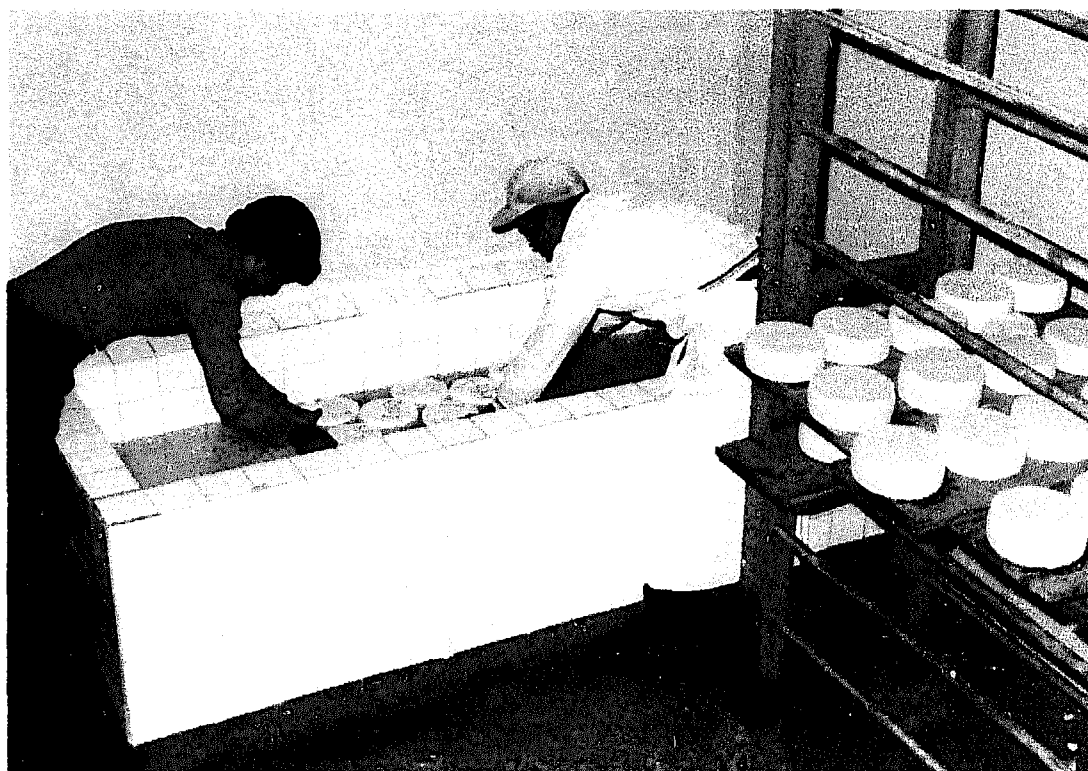
Photo 6. Tile-covered concrete brining tank (Nabuzo communal cheese plant).
